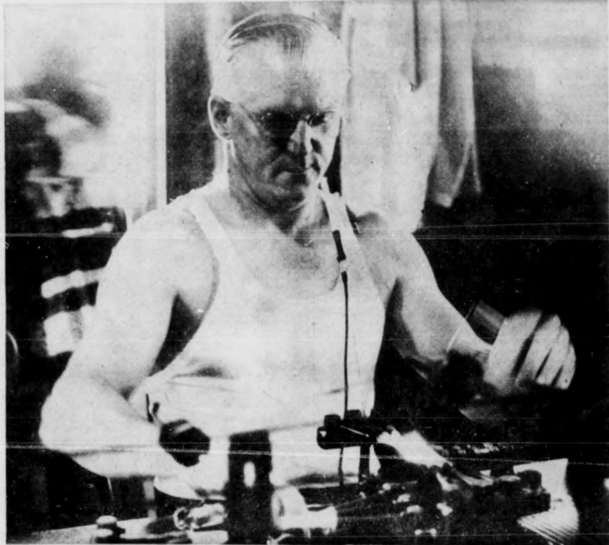
Charles Frost, 203 W. 11th Ave., Conshohocken, moves so rapidly with the heating device for glass, that the Recorder photographer is hardly able to snap picture. Frost is tooling glass ball bottom floats for some of the precision glass instruments,
