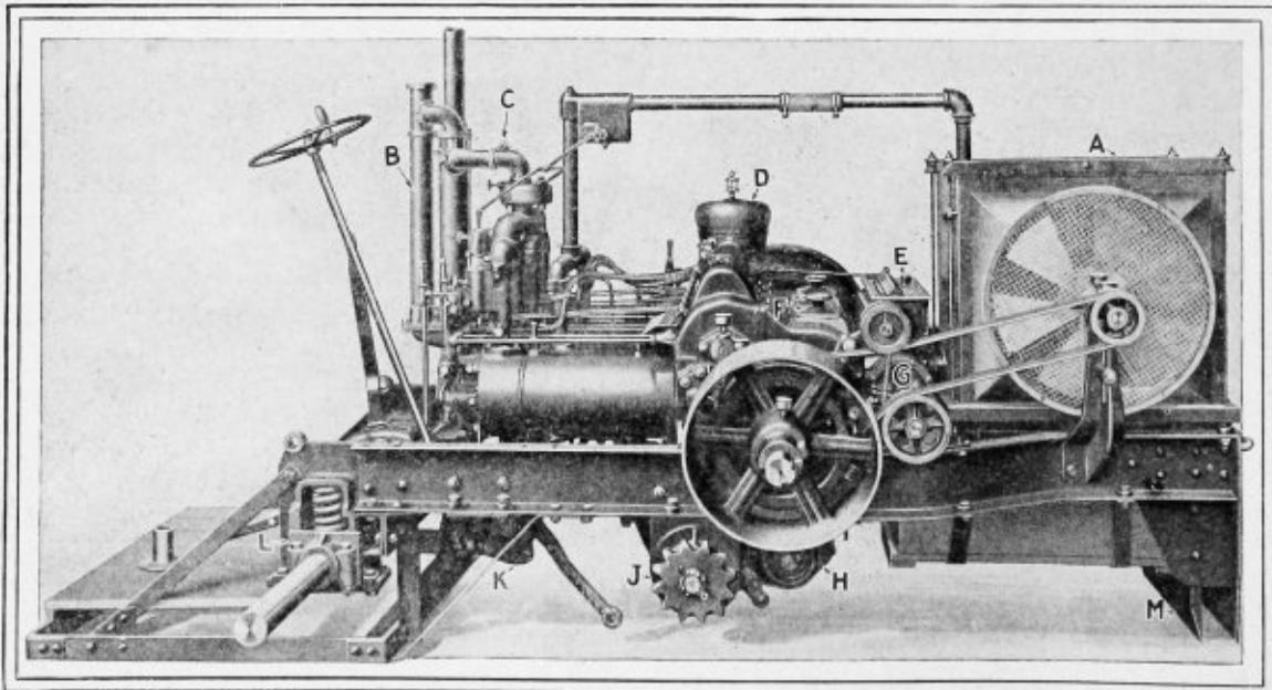
Engine Cooling System, Frame, and Platform of International 15-30
