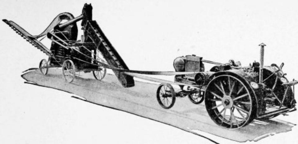
Furnishing belt power for a John Deere Corn Sheller--no gears in mesh at belt work
