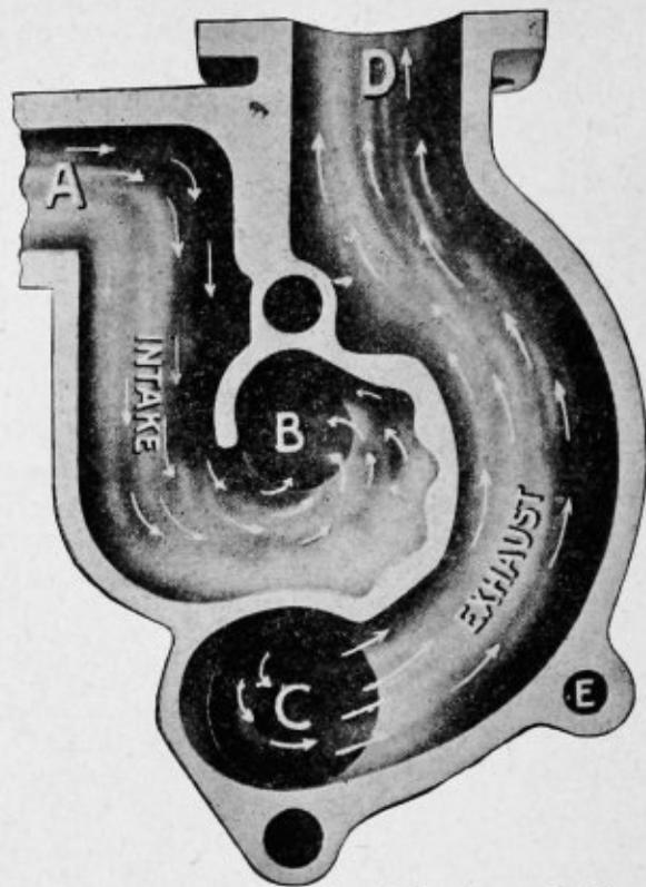
Cross Section of the Avery Gasifier—the Device that Does the Trick. Turns kerosene or distillate into gas and burns it all.
