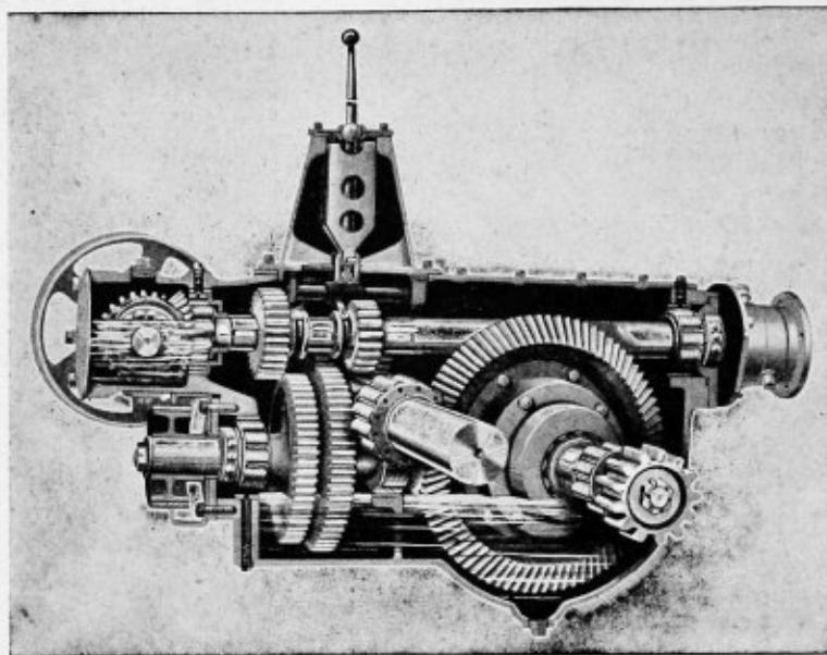
The Combination Bevel and Spur Gear Type Employed on the E. B. 12-20
