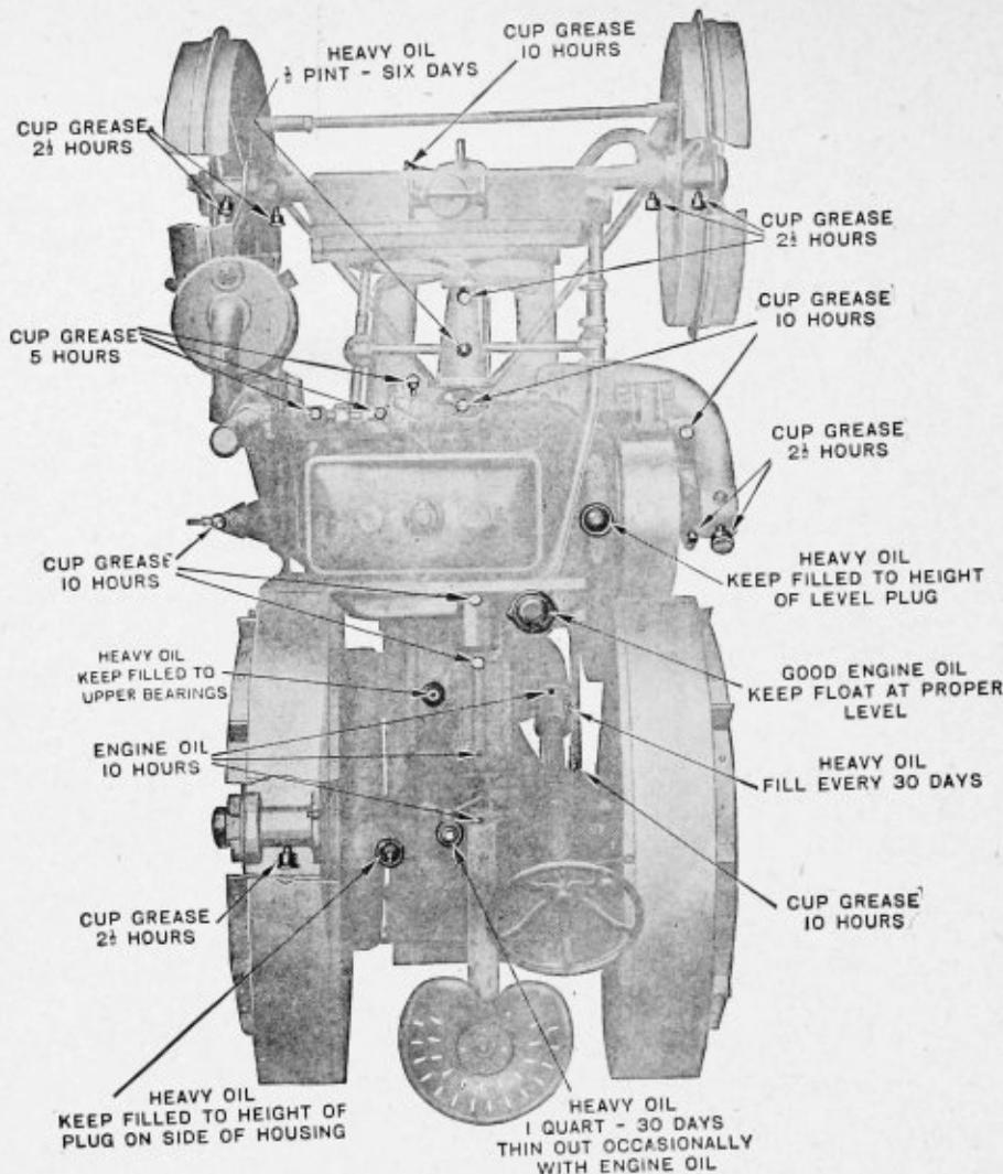
bull pinion and master gear. The illustration shown on this page clearly illustrates this housing which is oil tight.
