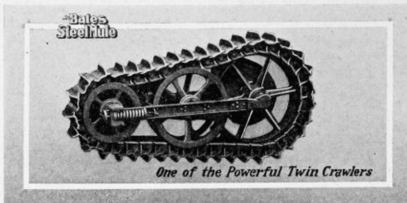
steel crawler connecting pin passes through this bushing as well as through the adjoining shoe. The pin has a key head so it cannot rotate in the shoe and makes all movement come inside of the hardened bushing.
