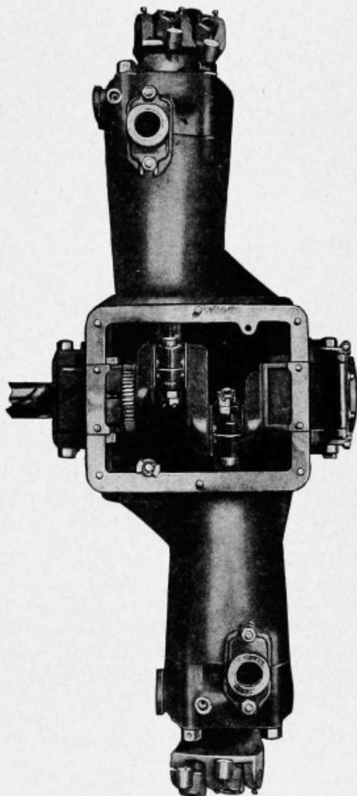
Top View of Two-Cylinder Avery Perfected Opposed Motor as Used in the Avery 8-16 and 12-25 H. P. Tractors.
