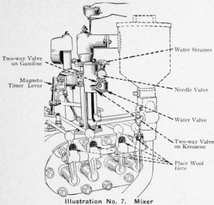
7. Open needle valve to marked position.
