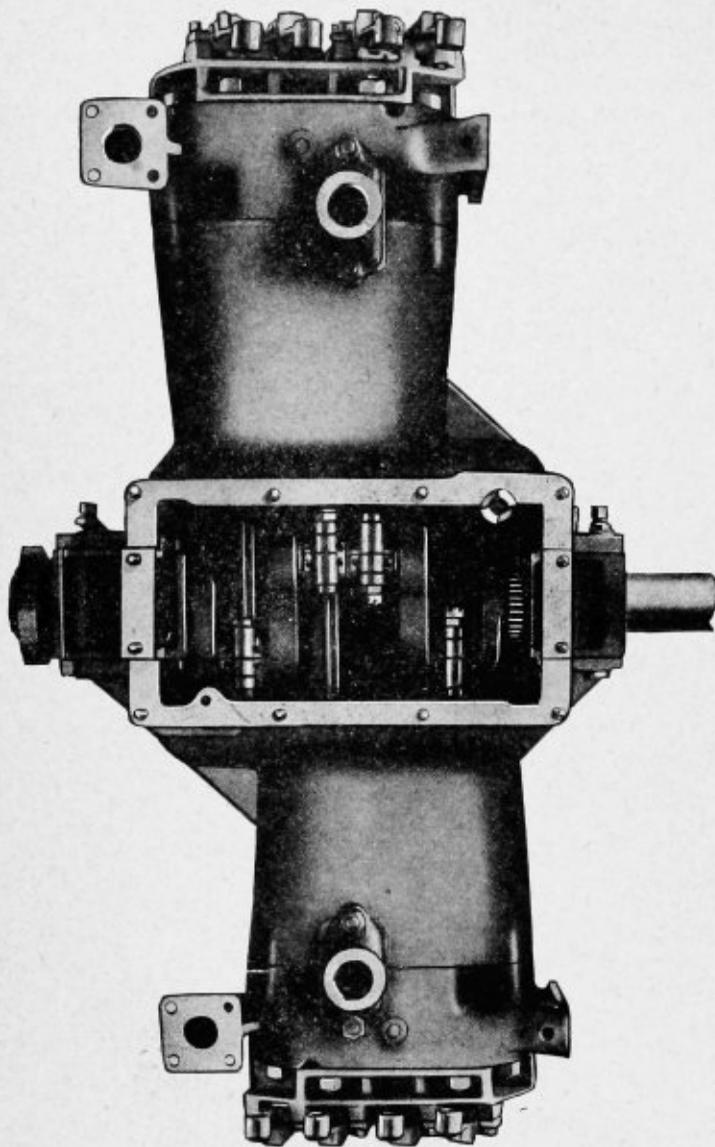
Top View of Four-Cylinder Avery Perfected Opposed Motor as Used in the Avery 14-28, 18-36, 25-50 and 40-80 H. P. Tractors.
