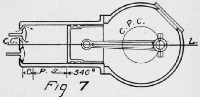
inder drops slightly below atmospheric as shown in Figure 6. During this stroke a new charge of gas enters the cylinder and continues to enter until the piston has reached the second out center, 540° (see Figure 7).
