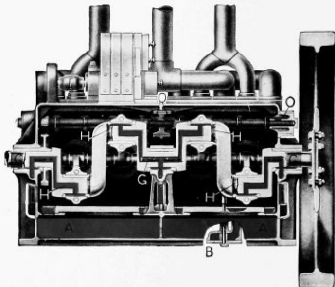
Application of Sediment Basin and Oil Grooves
