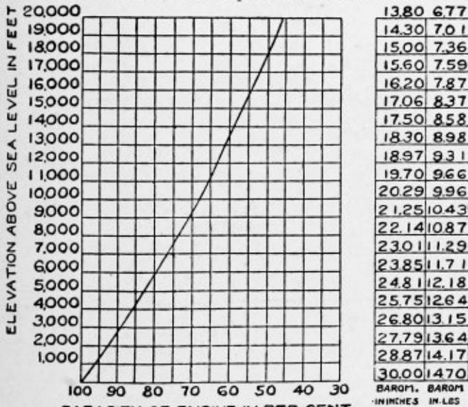
EFFECT OF ALTITUDE ON AIR PRESSURE AND GAS ENGINE HORSE POWER
