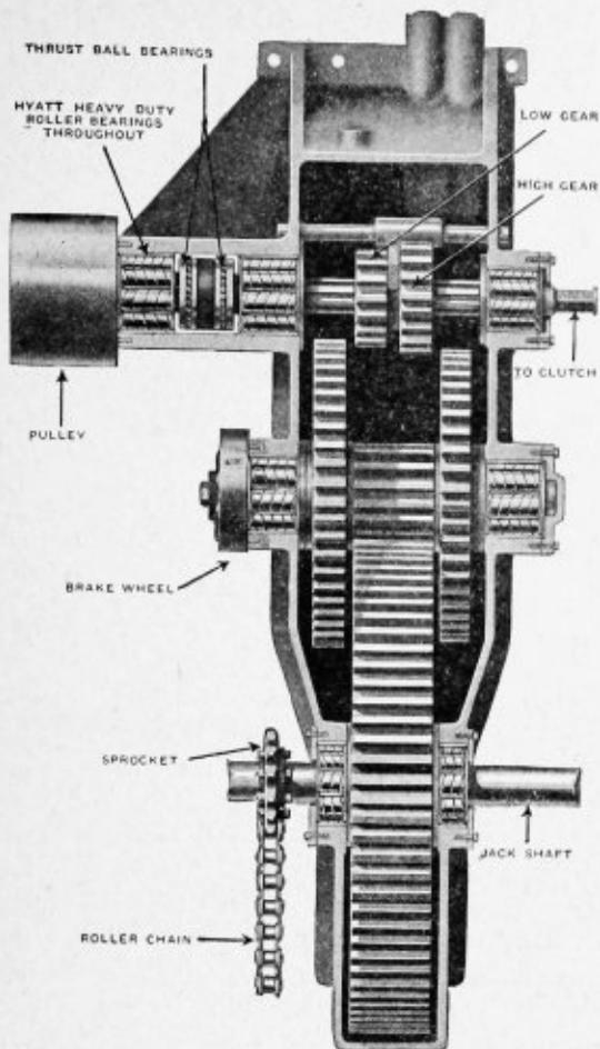
The entire transmission is mounted in one case which absolutely insures that all gears be kept in line, that they will mesh properly and that they will transmit power with the smallest possible wear and its attendant friction loss.
