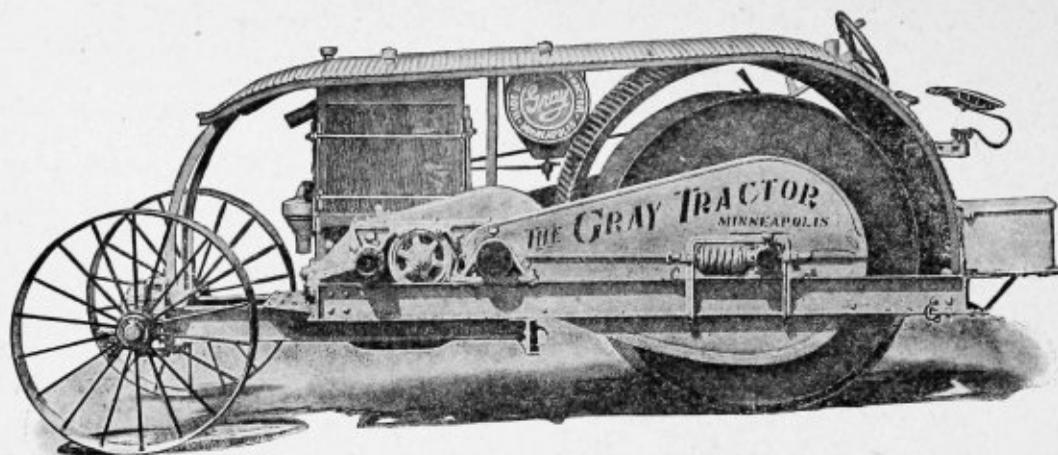
Then it is carefully fitted throughout. The two sides are drilled, and then reamed out true to size. In these sides are fitted hardened steel bushings, which are reamed and ground to size. **Hardened steel rollers run over these bushings and on the sprockets.** This construction gives a rolling contact, and reduces friction to a minimum. It also gives large bearing surface so that all danger of wear or stretch is eliminated. Through the nickel steel bushings run hardened nickel steel rivets.
