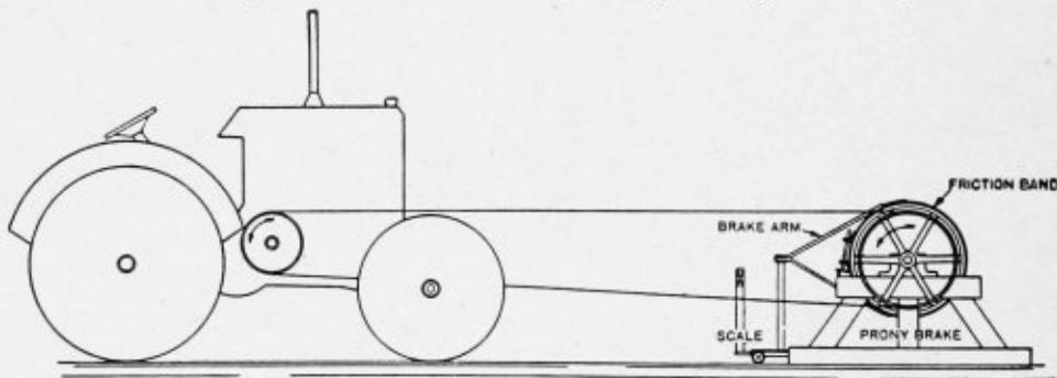
**Use of Prony Brake in Determining Brake Horse Power**
