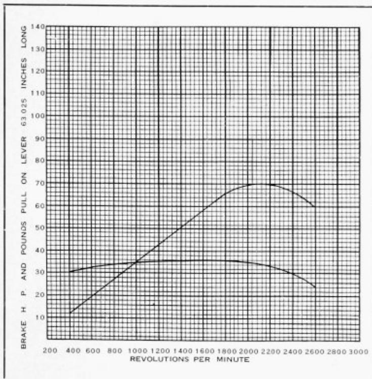
The figures along the left-hand edge of the chart, reading from the bottom up, show the horsepower developed. The Horizontal figures at the bottom, reading from left to right, show the number of revolutions per minute or the speed of the motor.
