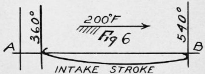
exhaust valve closes, the piston starts on the third or intake stroke.
