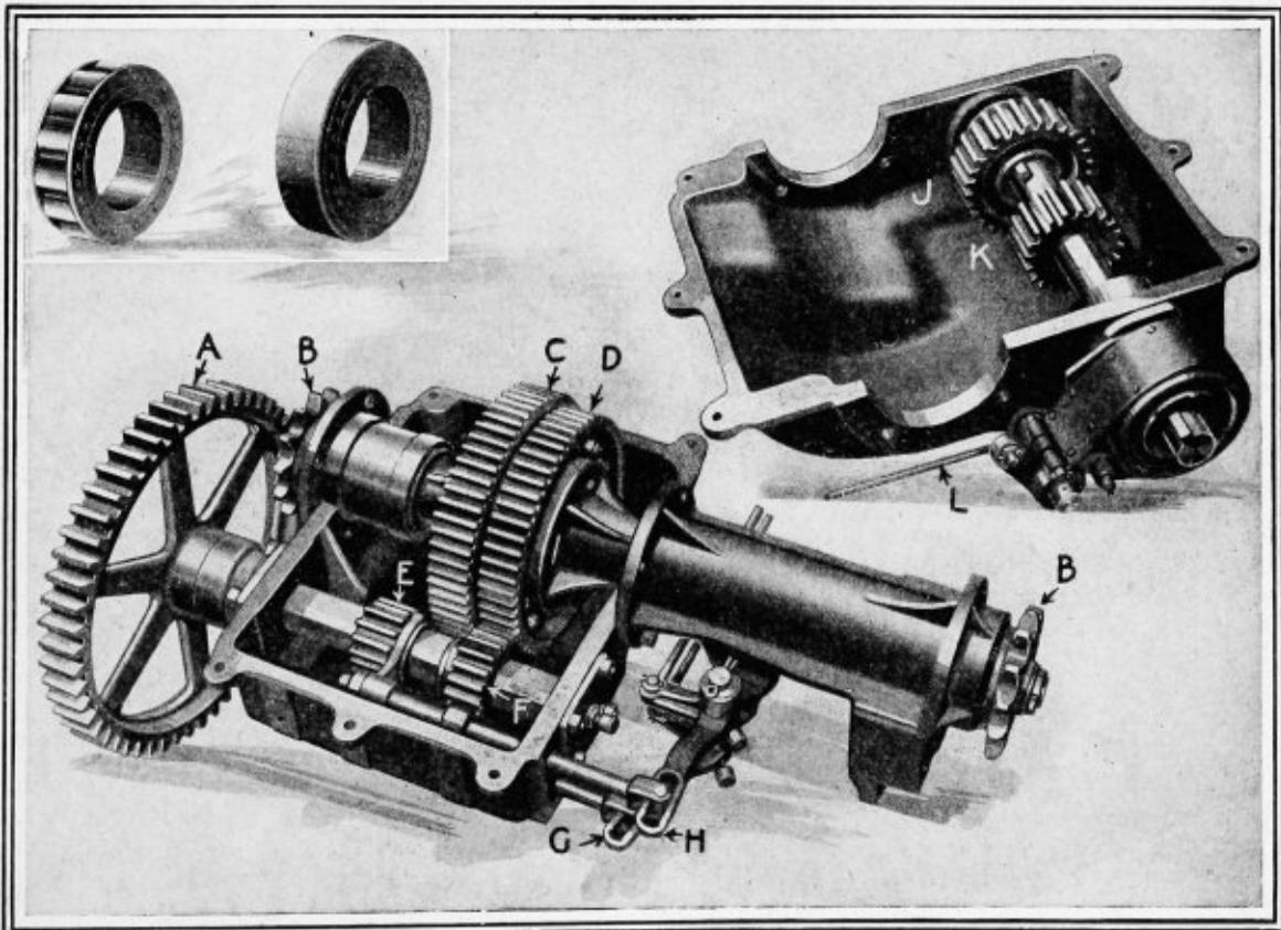
The transmission gears are entirely enclosed and run in oil. The principal bearings are roller bearings, as shown in the upper left hand corner
