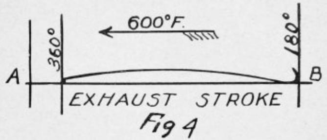
**18. The Exhaust Stroke.** At this point the exhaust valve opens as shown in Figure 3 and the piston starts on its second or exhaust stroke, the crank traveling
