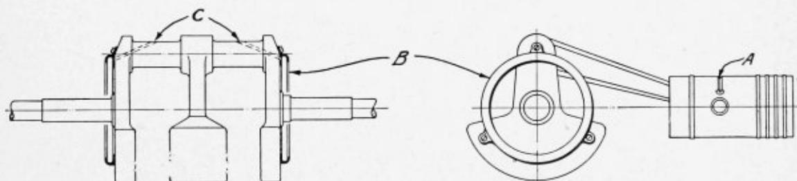
**The Madison Kipp Direct Lubricator, Installation, on a Twin Cylinder Horizontal Motor**
