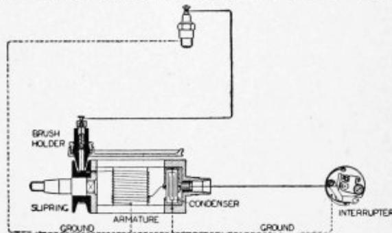
Circuit Diagram Type DU1 Bosch Magneto
