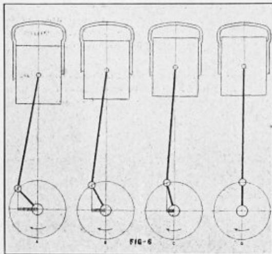
Position C shows the engine in operation with a hot, powerful high tension magneto spark, which is occurring still nearer dead center, wasting less fuel, generating more power in the forward or plus direction, and burning less fuel and exerting less power in the minus direction.
