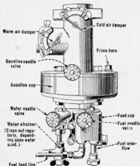
line supply for all cylinders, but in order to get the best results, there is a separate needle valve for kerosene for each cylinder. This gives a close adjustment and enables the owner to get the greatest economy of fuel and the most even operation. The water valve is automatic after once being opened and needs no special adjustment. See E, Illust. 10.
