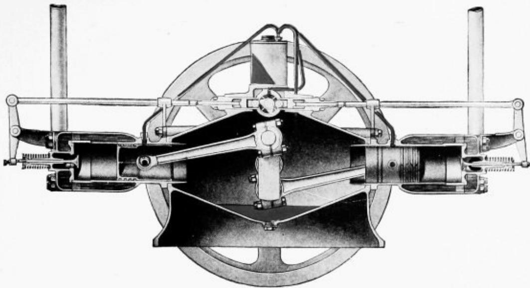
SYSTEM 11—SEPARATE FORCE FEED HORIZONTAL TYPE MOTOR
