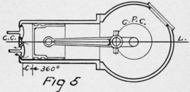
from 180° to in center at 360°. This is the exhaust stroke (see Figure 5.) The pressures in the cylinder are shown by Figure 4. At 360° or soon after the
