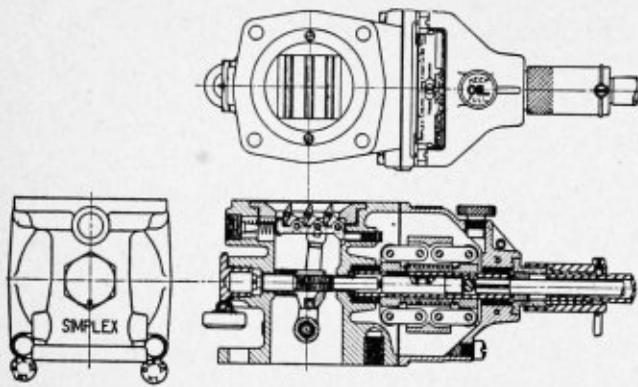
DETAILS OF A GOVERNOR FOR TRACTOR ENGINES IN WHICH THE MOTION OF THREE SHUTTERS THROUGH AN ANGLE OF 60 DEG. PROVIDES THE CONTROL OF THE THROTTLE-VALVE
