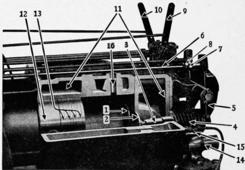
The intake and exhaust valves are opened and closed mechanically by means of cams on a cam shaft operating through the valve gear. The relative timing of the valve movements is regulated accurately when the engine is built. Re-timing is necessary only after the crank shaft or cam shaft has been removed. The operator, by carefully following printed instructions can do the re-timing himself.
