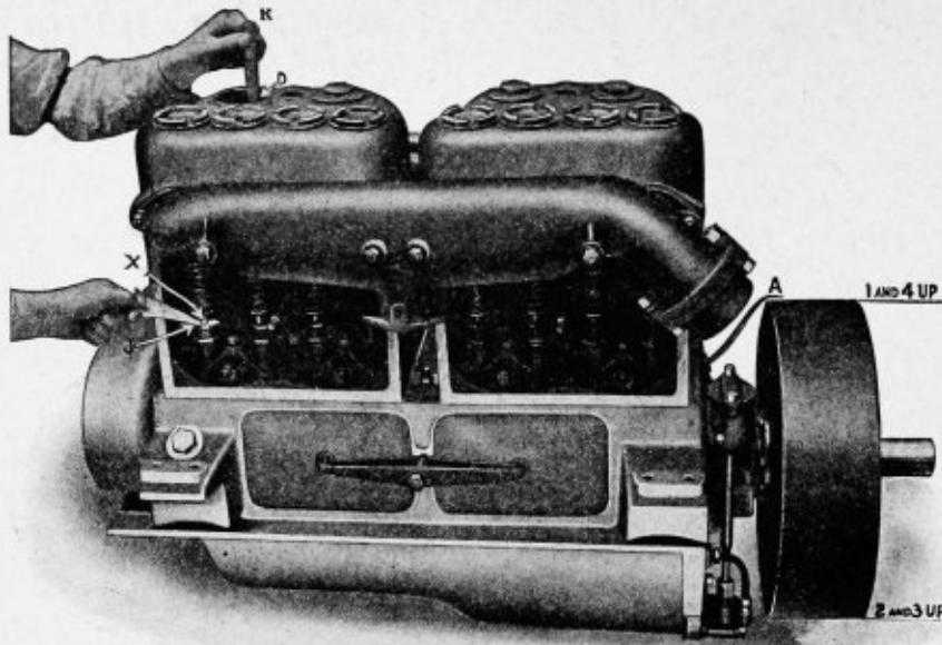
As a rule Waukesha Motors have their flywheels marked as to when the valves should open. The following method is applied in case the flywheel and the timing gears are not marked.
