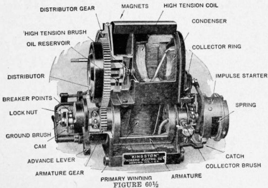
that brass plate on distributor disc is directly underneath the terminal on distributor head, which you will use for cylinder No. 1. See that wires are placed on terminals in the firing order of your motor. Be sure that you place wires on distributor head in opposite direction to rotation of armature.
