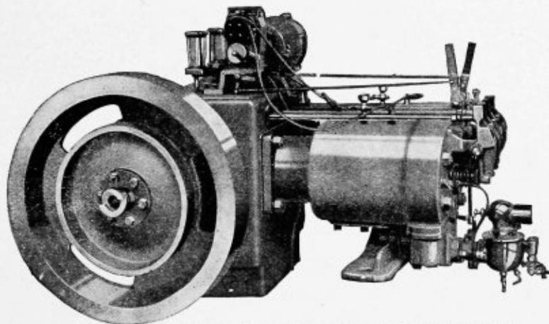
Flywheel side of Waterloo Boy's kerosene burning, non-vibrating motor
