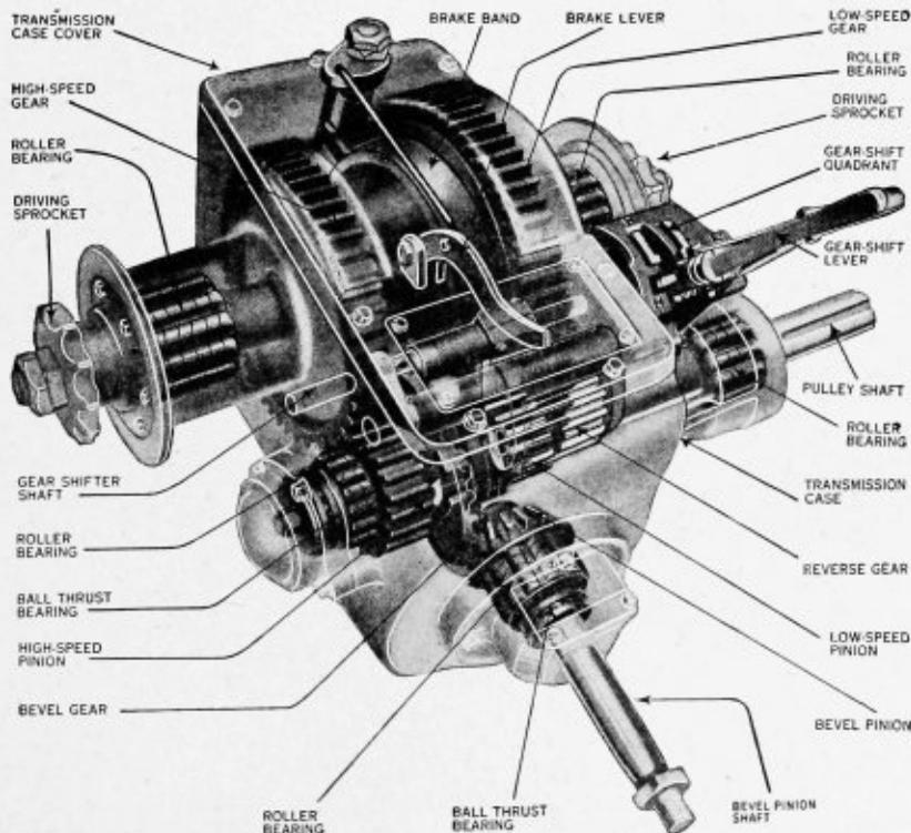
The Combination Bevel and Spur Gear Type Employed on the Nilson Tractor
