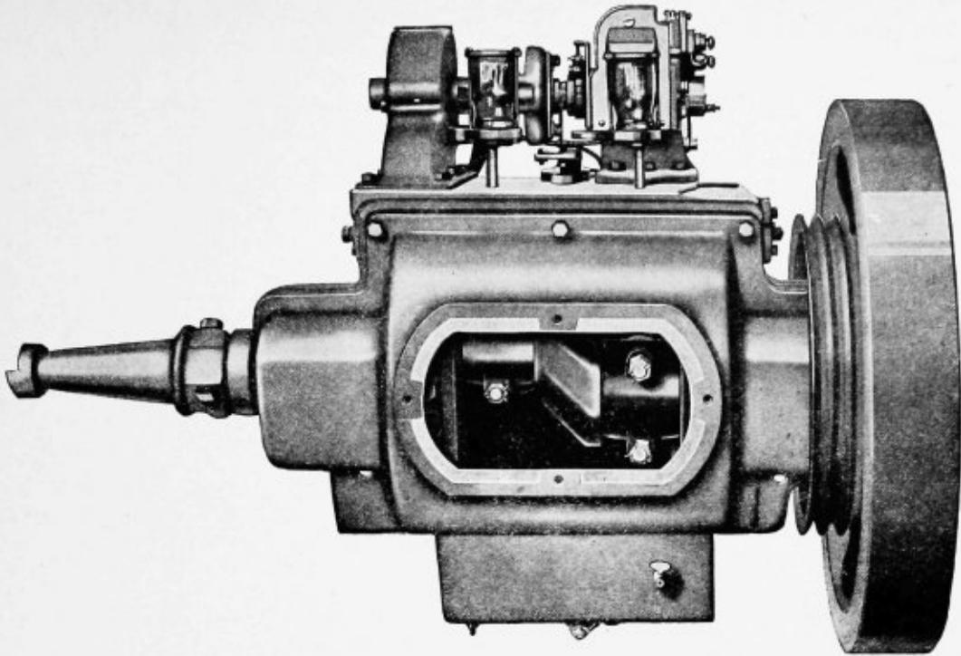
Crank Case View of Motor with Inspection Plate Removed
