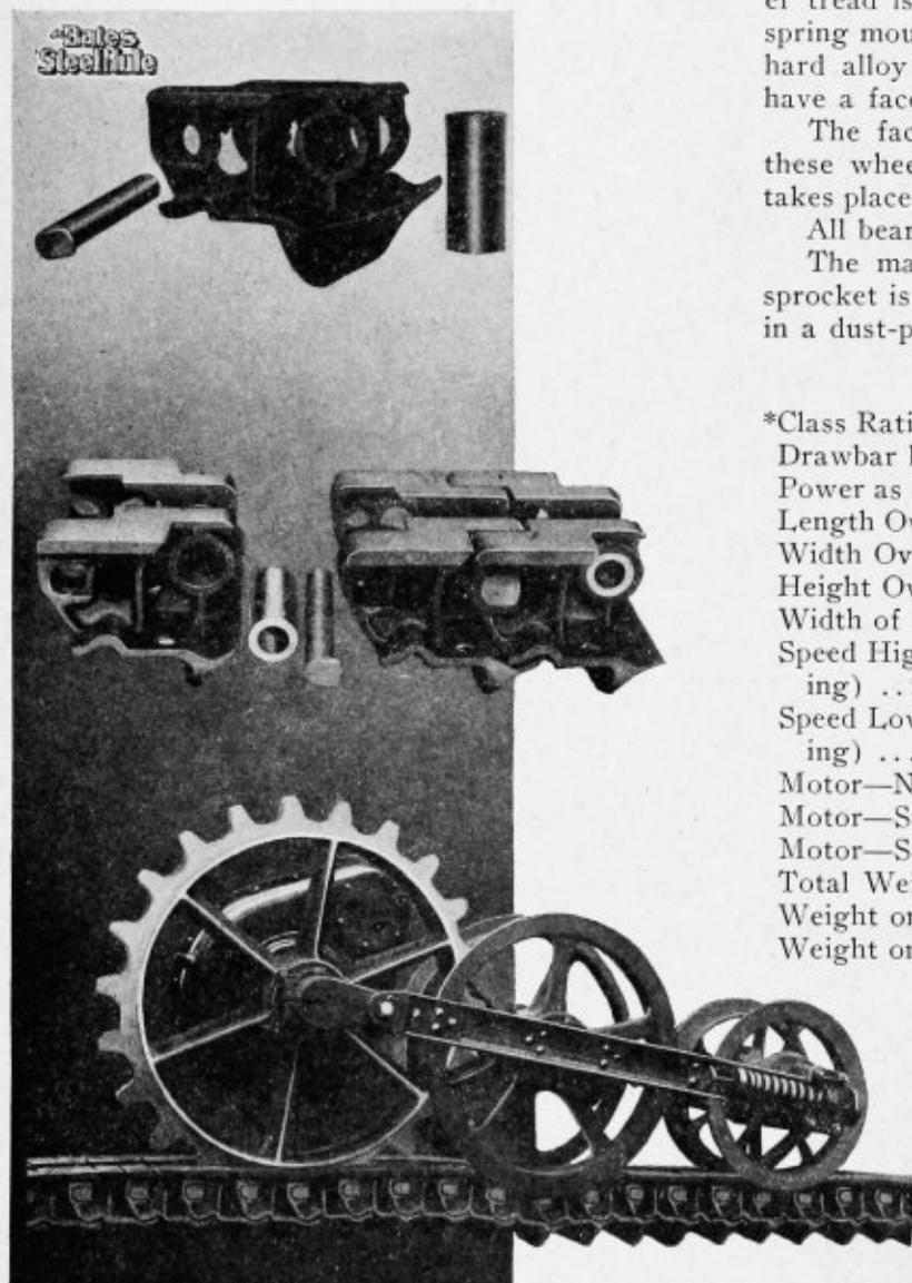
tion to their work and the resultant wear is therefore very slight. If after several year's service it is desirable to renew the crawler wearing parts, new bushings and pins can be purchased at a nominal price and inserted very easily.
