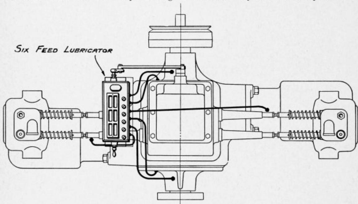
**The Madison Kipp Direct feed Lubricator, Installation, on a two cylinder horizontal opposed motor.**
