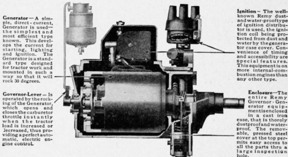
**Generator**—A simple, direct-current, Generator is used—the simplest and most efficient type known. This develops the current for starting, lighting and ignition. The Generator is a standard type designed for tractor work and mounted in such a way so that it will rock 30 degrees.
