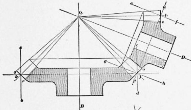
ANGLE OF AXES LESS THAN 90°
