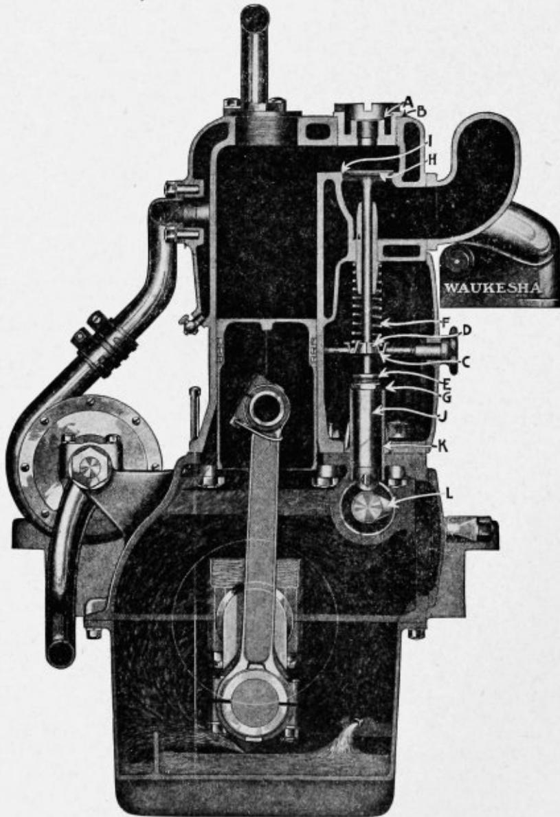
Sectional End View of Waukesha Motor, showing Operation and Interior Construction. Note how the drip of the connecting Rods causes a spray of oil to circulate, thoroughly oiling every bearing of the Crank Shaft, the Cam Shaft the Push Rds, Pistons and Piston Pin Bushings. Note how the oil vapor circulates past the push rod and up into the Valve Case Chamber.
