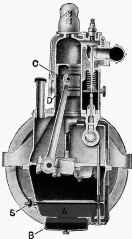
Application of Sediment Basin and Oil Grooves.
