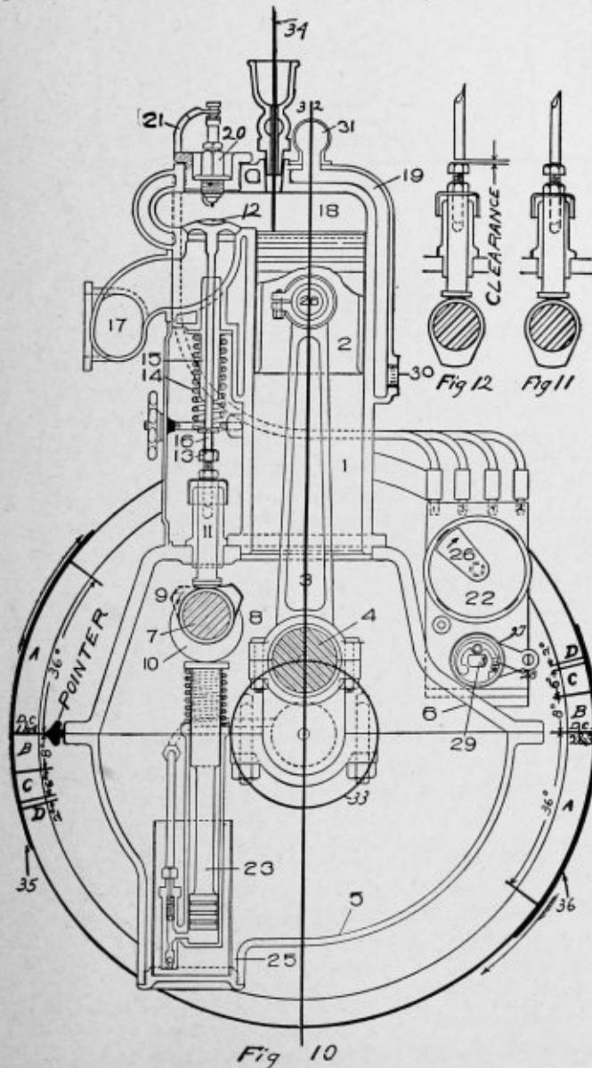
Since the position of D. C. in the motor marks a convenient starting point from which to calculate the time of the occurrence of various phenomena in the operation of a motor, it is necessary to become familiar with rules for determining the position of this point.
