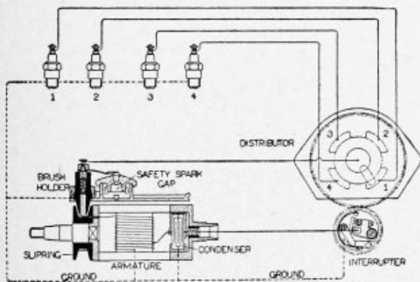
Circuit Diagram Type DU4 Bosch Magneto
