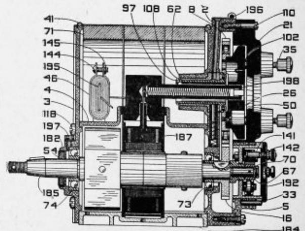
Cross Section Model T Magneto
