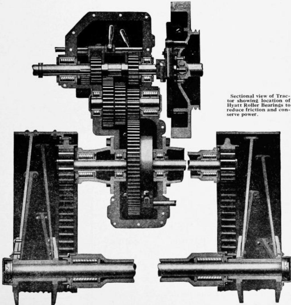
Sectional view of Tractor showing location of Hyatt Roller Bearings to reduce friction and conserve power.
