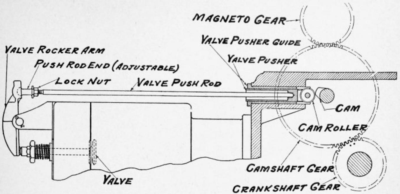
justed by loosening the lock nut on rear end of valve push rod and screwing into or out of the valve push rod adjuster. Shortening the rod causes the valve to open later and close earlier, while lengthening rod opens valves earlier and closes it later.
