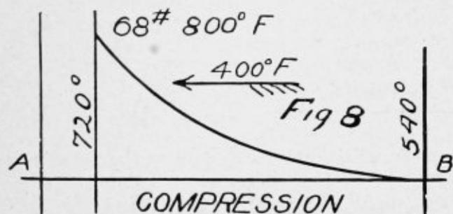
the piston again reaches 720° or zero degree, dead center, as shown in Figure 1, and the cycle is renewed second and third time, and so on, continued indefinitely.
