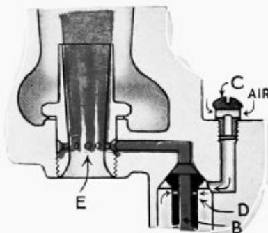
The gasoline, leaving the float chamber past the point of the high speed adjusting needle, rises through a vertical channel "B." Air taken in through the "Air Bleeder" or protecting cap "C," discharge into the gasoline channel through small holes "D," breaking up the flow and producing a finely divided emulsion. This then issues forth through a number of jets into the high velocity air stream of the small venturi "E."
