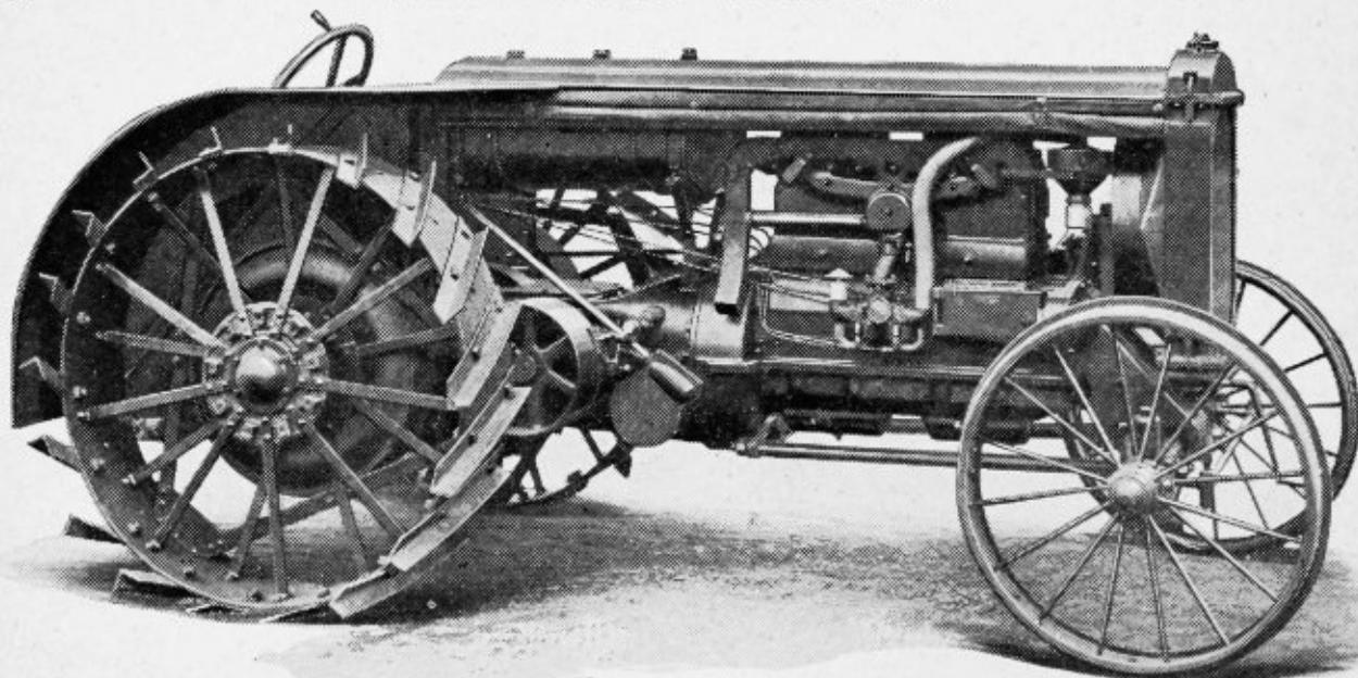
The motor is equipped with a Kingston double bowl carburetor being fed by gravity and a high tension Eiseman Magneto with an impulse starter.
