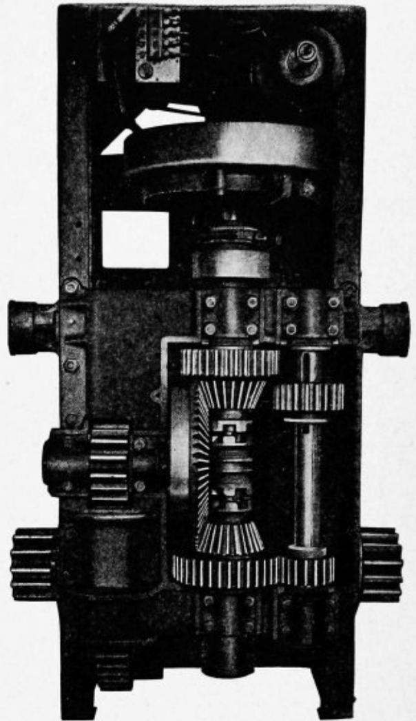
The Combination Bevel and Spur Gear Type Employed on the Twin City 25-45.
