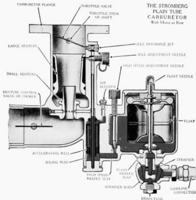
A Plain Tube Carburetor is one in which both the air and the gasoline openings are fixed in size; and in which the gasoline is metered automatically, without the aid of moving parts, by the suction of air velocity past the jets.
