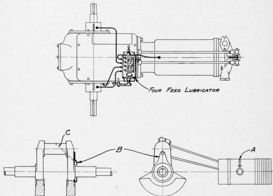
**The Madison Kipp Direct feed Lubricator, Installation, on a single cylinder horizontal motor.**
