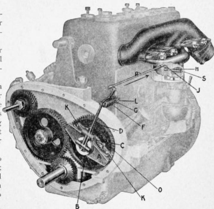
"L." Turning "L" in direction indicated by arrow causes motor to speed up, while turning "L" in opposite direction causes motor to slow down.
