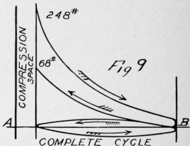
Owing to the rapidity of the movement of the piston it is impossible to have the exhaust valves or intake valves large enough to prevent this positive and negative pressure, but on a poorly designed motor we have more positive pressure during the exhaust stroke and more negative pressure during the intake stroke. The greater these curved lines vary from the straight line A-B, the greater the loss in power during these strokes and the less efficient the motor.
