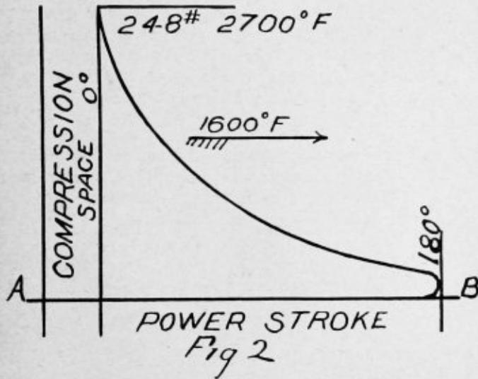
At this point ignition takes place and ignites the charge in the gas motor cylinder which
