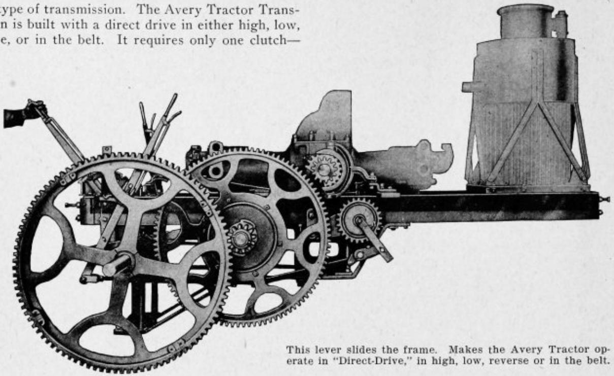
This lever slides the frame. Makes the Avery Tractor operate in "Direct-Drive," in high, low, reverse or in the belt.
