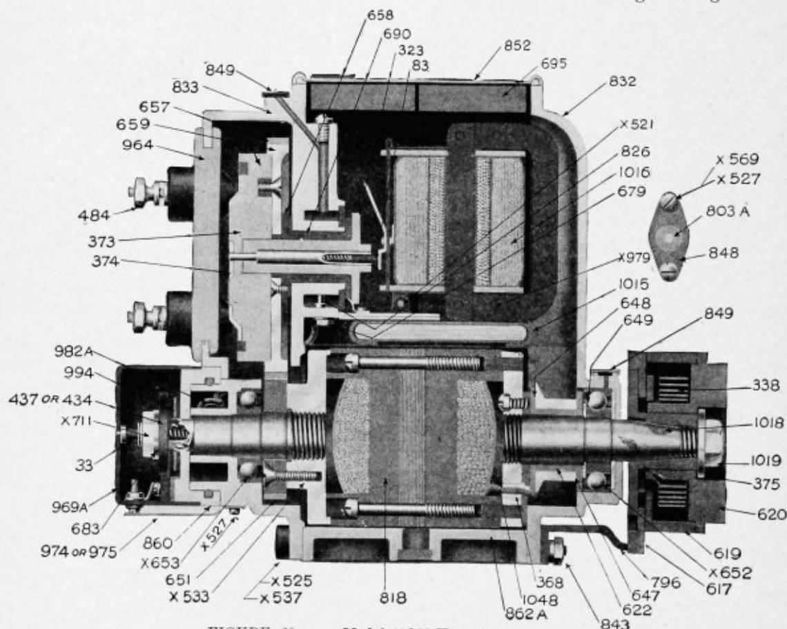
FIGURE 60 Model "O" Kingston Magneto with Impulse Starter
