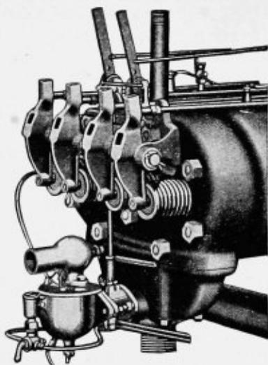
View showing close connection of carburetor, manifold and cylinder head. Note that the patented manifold is a combination of the exhaust and intake.
