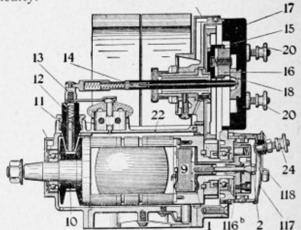
Longitudinal Section of DU4 Magneto
