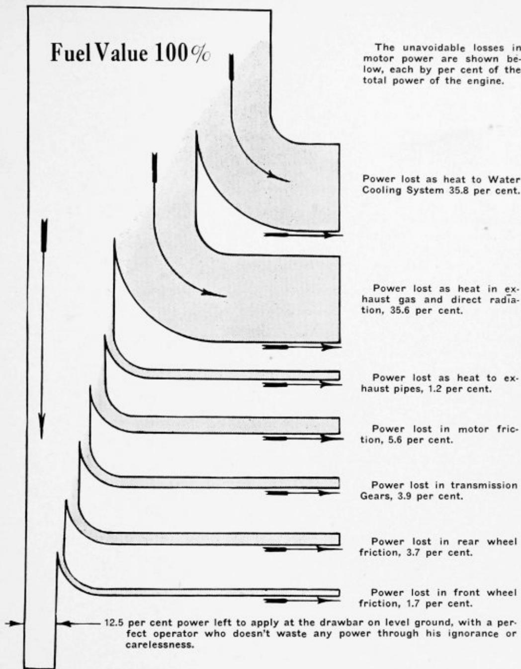
From Fig. 1 we see that only 12.5 per cent of the total energy in the fuel consumed is left for useful work at the drawbar on level ground: and in soft fields, or hills, the loss is still greater.
