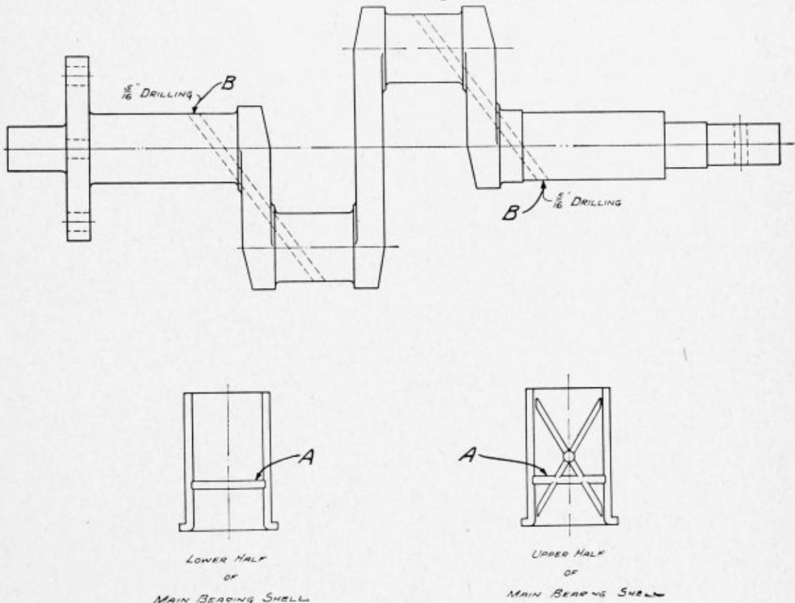
Also a type of crank shaft arrangement and bearing grooving for conducting surplus oil from main bearings to crank pins.
