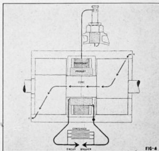
Instead, however, of a storage battery we have permanent magnets. The permanent magnets in this view are not shown, as we are looking up from the bottom of the magneto so as to get a better view of the windings and core.
