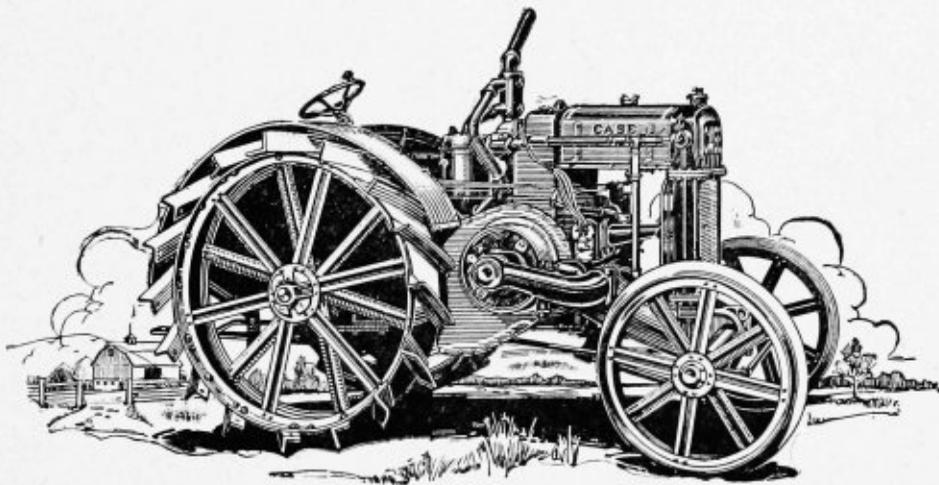
tough soil or on grades or four plows under favorable conditions. Naturally this tractor will do any other drawbar work requiring similar power. At general hauling it will pull from 10 to 15 tons, depending upon grades and footing.
