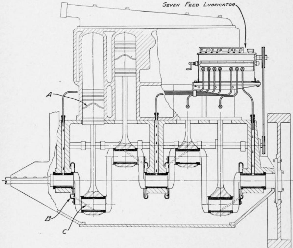
**The Madison Kipp Direct feed Lubricator, Installation, on a Four Cylinder Vertical Motor.**
