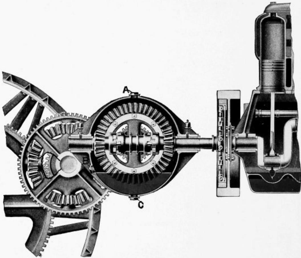
FARM TRACTOR TRANSMISSION AND DIFFERENTIAL LUBRICATION
