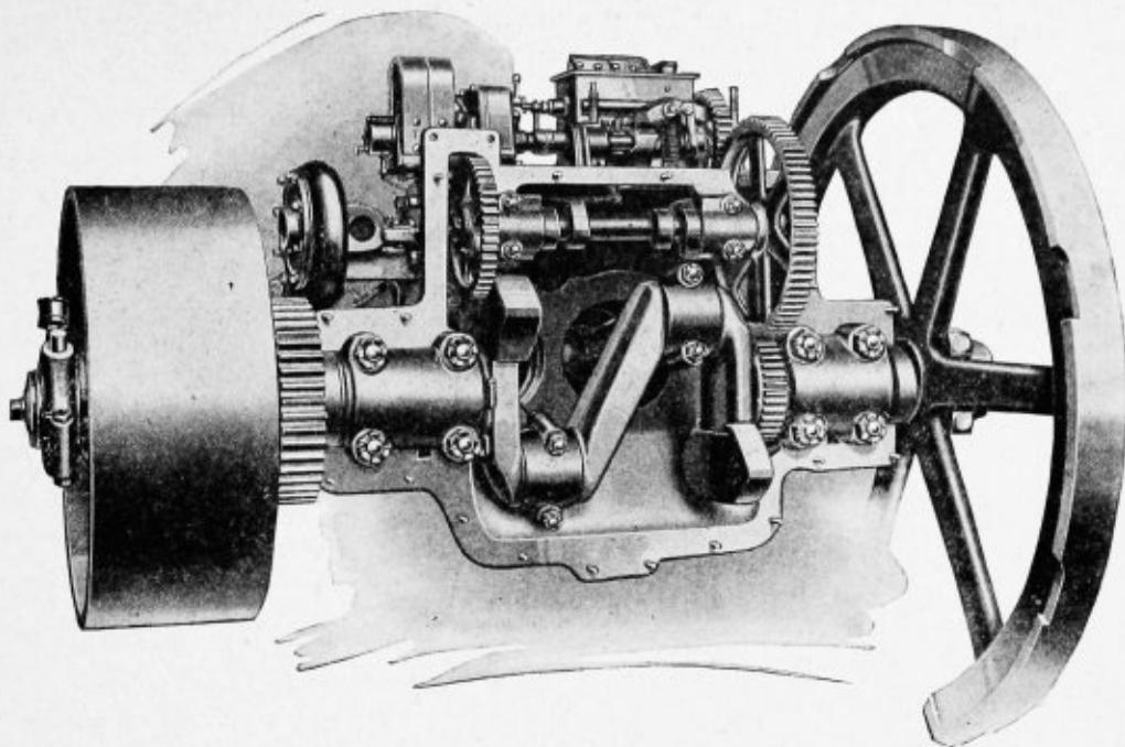
"16-30" Motor with Crank Case Cover Removed
