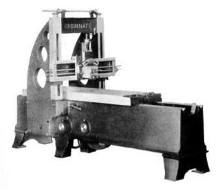
The shifting mechanism has been greatly simplified. A barrelshaped cam, rigidly supported between two bearings, has been substituted for the straight or circular cam.
