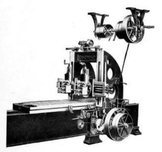
With this machine in operation two speeds are acquired— The right speed for roughing.
