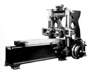
Instead of straight gibs, taper gibs have been provided and the vertical slide is provided with ball bearings to facilitate easy handling.
