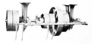
The illustration shows the arrangement—two belts from the line shaft similar to what we now have, except that we included the same idea which was formerly associated with our gear box; that is to say we began with a friction clutch.
