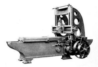
This original machine, the first we ever built, had straight gibs. The vertical slide was without ball bearings.
