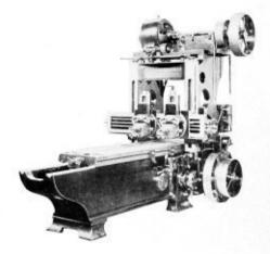
The above picture shows the first planer we ever made arranged with a variable speed transmission giving a constant return. This is in the form of a gear box having a gear transmission very much similar to that of an automobile gear case, except that the speeds were selected by the handles shown at the side of the housings, which operated friction clutches.
