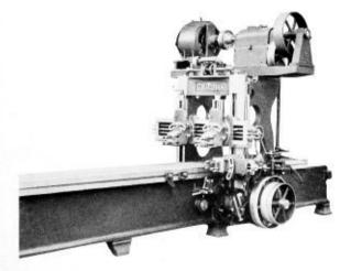
Despite the fact that in our old design we made the friction clutches for selecting the speed variations large and adjustable, we could not find a clutch that would stand up to the service.
