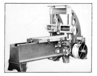
The increased stability received from placing additional legs near the middle of the bed goes to make remarkable production records.
