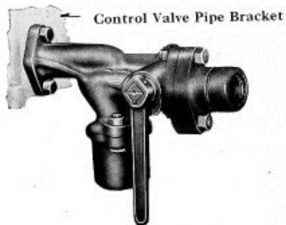
Fig. 25. Combined Dirt Collector and Cut-out Cock with Reinforced Flanged Union
