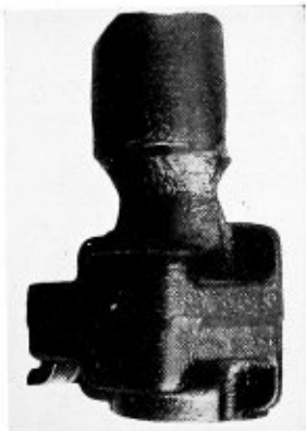
In foundries sinkers are removed by using the carbon electrode process.
