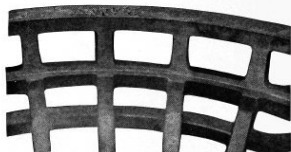
Blow holes developed in this large casting during machining. The holes on the left have been chipped and cleaned for Electric Welding. Completed welds are shown at the right before being remachined.
