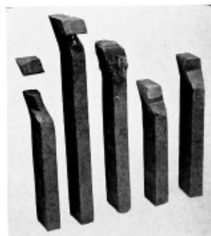
Lathe tool made by welding high speed steel tip to shank of low carbon steel.
