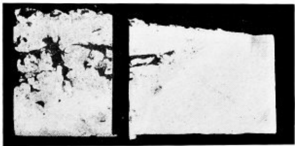
Cross sections of weld made with Norway iron electrodes, showing slag content caused by excessive oxidation characteristic of very low carbon electrodes.
