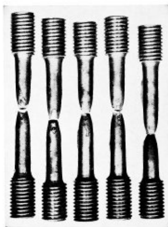
Negligible effect of striking an arc on the physical characteristics of mild steel.
