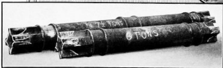
Wobblers saved from the scrap heap by building up worn ends with the electric arc.
