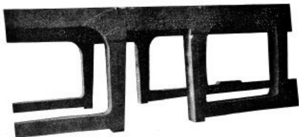
A fractured locomotive frame repaired by means of the Electric Arc.
