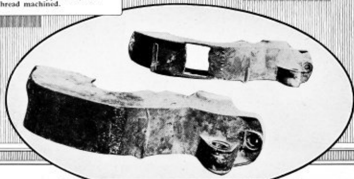
Upper view, worn gear case. Lower view, gear case with similar hole patched by Arc Welding.
