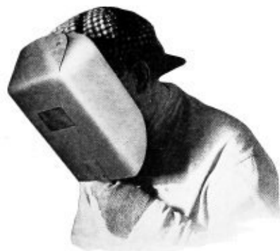
Operator holding shield.
