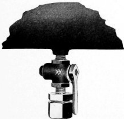
Fig. 13. Showing Orifice Disc Holder Screwed into Main Reservoir Drain Cock
