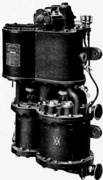
Fig. 1. 8\frac{1}{2} -Inch Cross Compound Compressor, Air Inlet Side
