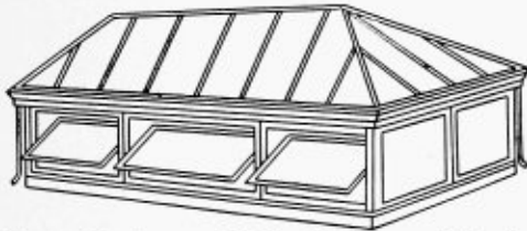
No. 9 Monitor with Hip Skylight and Ventilating Sash
