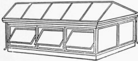
No. 5 Monitor with Double Pitch Skylight and Ventilating Sash
