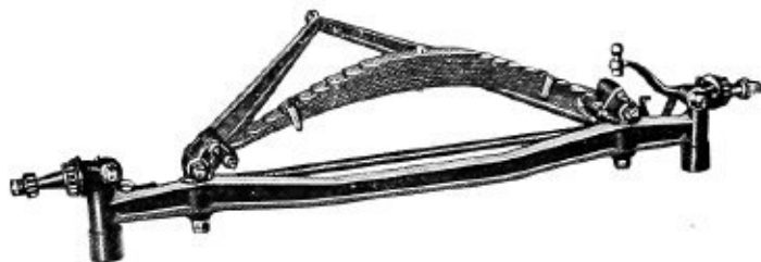
Inequalities in the road are easily cared for by this efficient type of front spring construction.
