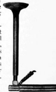
Exhaust valve cutting piece of cold-rolled steel shafting.
