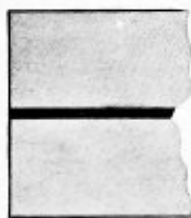
Fire Clay joint before firing.
