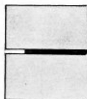
After firing. Fire Clay joint open, allowing heat to attack front surface and portions of sides of brick.
