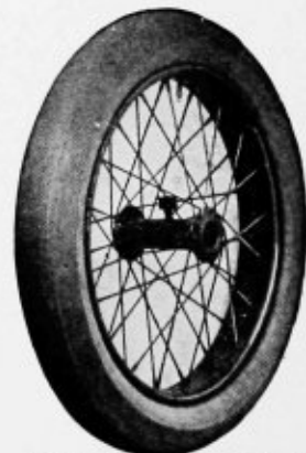
J N 4 Aeroplane Wheel For Curtiss Training Plane Tire Size 26" x 4" Plain Clincher
