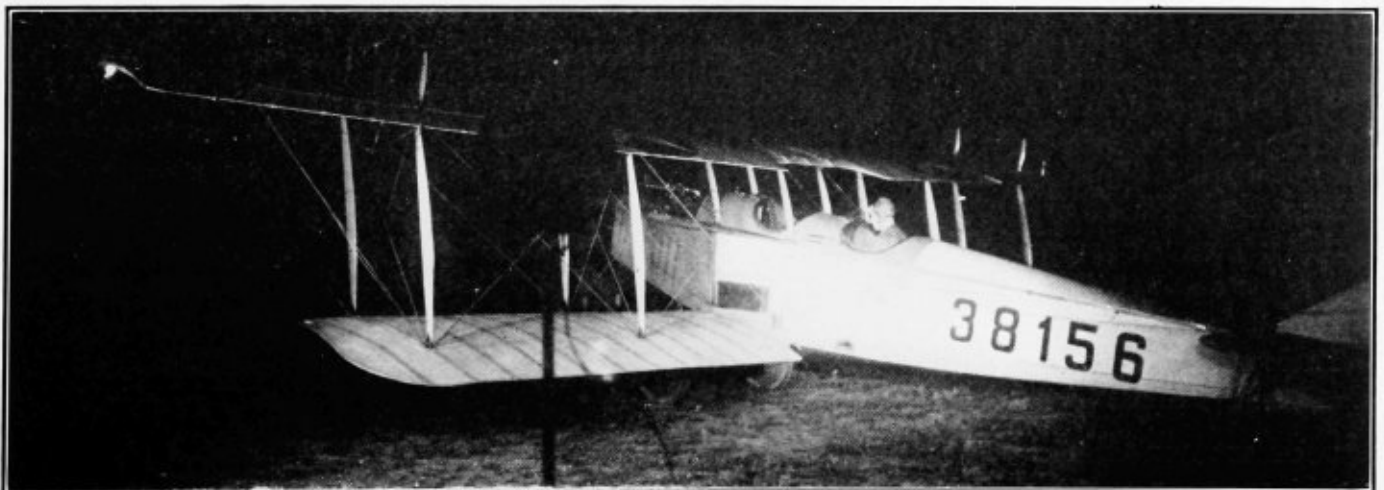
A night flying aeroplane. The floodlight lights up the ground to assist in landing the machine.
