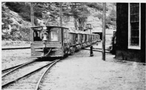
25-ton haulage locomotive pulling ore cars from underground tunnel to the mill of an Arizona copper company
