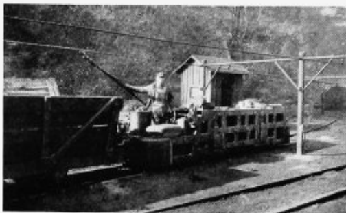
The maintenance expense of this 20-ton haulage locomotive operating in a West Virginia coal mine has been carefully watched and found to be extremely low
