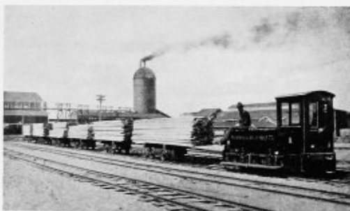
An industrial storage-battery locomotive used in yard haulage at the plant of a large Washington lumber company. There is no fire hazard with this type of locomotive
