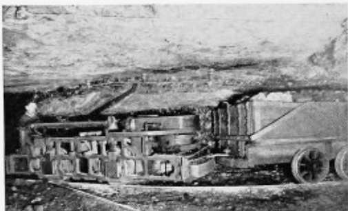
A 6-ton traction reel gathering locomotive is shown leaving the room neck with a loaded car in a West Virginia coal mine
