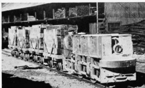
Barsteel storage battery locomotive, hauling mine timbers at a large Arizona copper mine. The location of the battery, together with the open frame construction, allows inspection without the necessity of removing the battery
