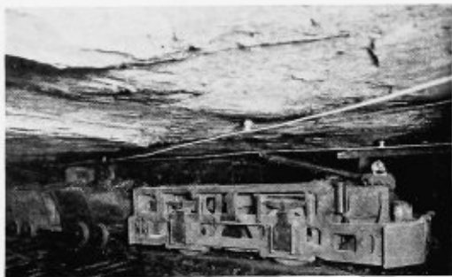
A 15-ton haulage locomotive in a western Kentucky coal mine. This illustration shows the solid construction of Barsteel locomotives
