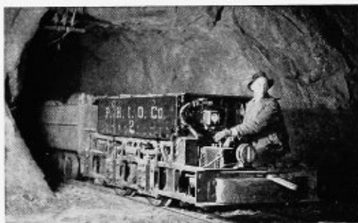
A Barsteel A6-2 storage battery locomotive in an iron mine in northern New York. This locomotive permits the battery compartment to be rolled off for charging
