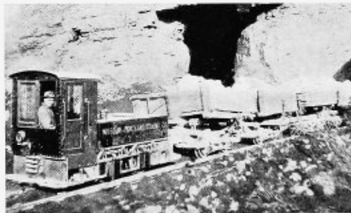
A storage battery locomotive equipped with end cab used for surface haulage at a quarry in Missouri. The cab is of plate steel with ample door and window space
