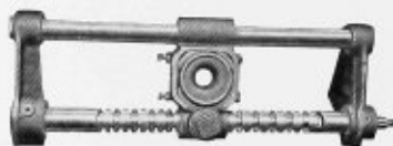
View of cable guide mechanism. A guide tongue fitting in the lead-screw at the bottom causes the guide to travel to and fro as the screw rotates
