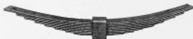
Typical leaf spring showing spring clip and the slots at the ends which hold the hangers
