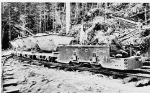
This old type Westinghouse-Baldwin haulage locomotive has been in continuous operation in Canada since 1900 and is still giving good service
