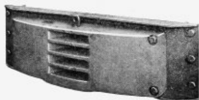
A standard built-up bumper permits easy coupling at various drawbar heights
