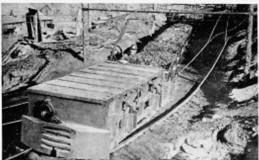
All-day service hauling heavy trips like this requires motor equipment with high continuous capacity. Locomotive in use at a West Virginia coal mine
