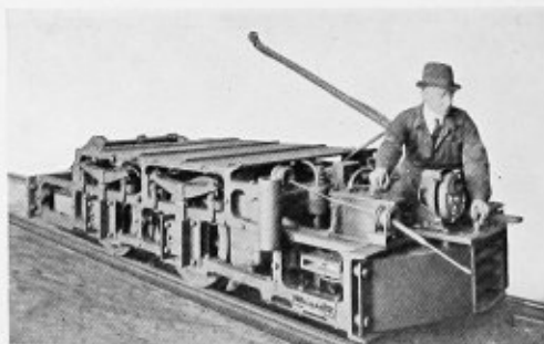
Equipment is so arranged in the operator's pit as to be within comfortable reach. The illustration shows how easily the locomotive can be inched and coupled
