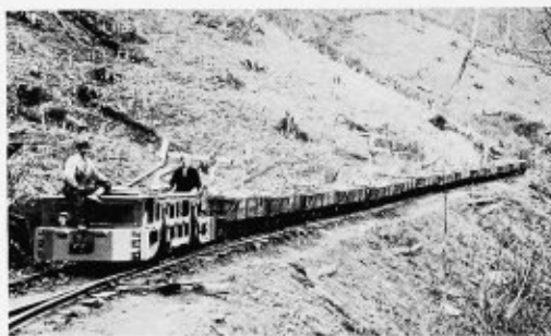
This locomotive has been in continuous operation for 14 years, hauling heavy loads up steep grades. Forced ventilation which increases the continuous capacity of the motors is particularly desirable here
