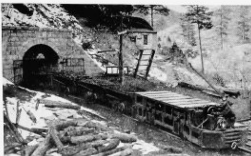
A 15-ton Barsteel locomotive hauling coal out of a drift mine in New Mexico. A feature of this type of locomotive is its low maintenance
