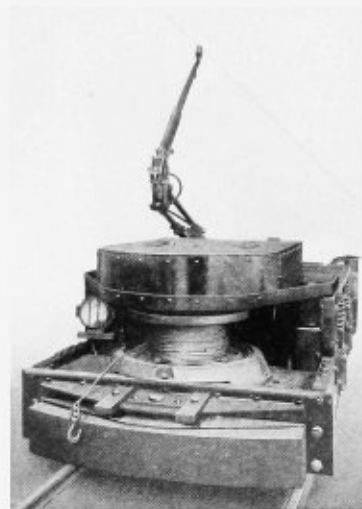
Rear view of standard gathering locomotive equipped with wire rope reel
