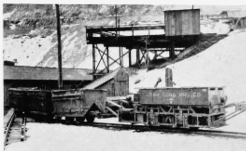
Standard storage battery locomotive equipped with special bumpers. These bumpers were made necessary by the special mine cars in use at this Utah copper mine
