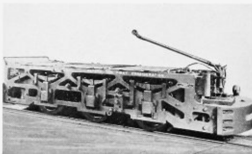
Standard 3-motor locomotive for heavy duty where track or gauge is too small to use 2-motor locomotive. Note that the springs are cross equalized
