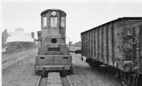
25-ton push-pole locomotive with air operated arms in use on lake ore docks. The use of these locomotives invariably results in relief from yard congestion and a saving in engine crew wages.
