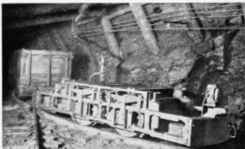
A 6-ton locomotive hauling cars in an anthracite mine in eastern Pennsylvania. The locomotive is equipped with a standard Westinghouse spring-supported headlight
