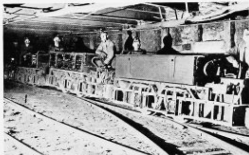
A group of locomotives in an Illinois coal mine. These locomotives are especially economical in power consumption for gathering work
