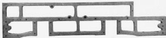
This illustration shows how the open Barsteel construction gives both strength and accessibility
