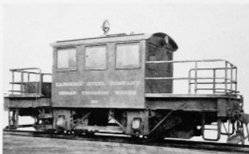
Special platform type locomotive with center cab, built for a Pennsylvania steel company. This locomotive is used for hauling ingots and semi-finished steel between departments
