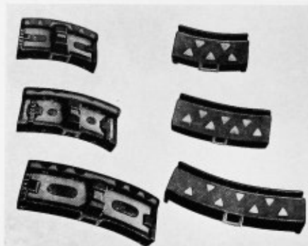
These steel-insert brake shoes of the MCB type prevent the shoes and wheels from wearing unevenly
