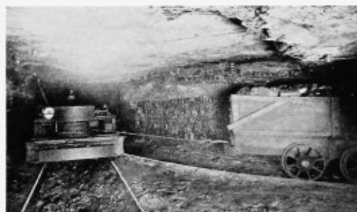
Gathering locomotive with traction reel pulling loaded car from room to cross entry, motor operated drum reeling in the steel cable
