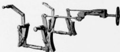
Skeleton view of brake rigging shows the direct positive action of brakes. Adjustment to offset wear on shoes is made by changing the leverage
