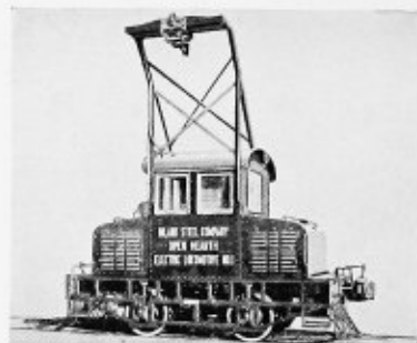
Special locomotive for an Indiana steel company used in yard haulage and inside buildings. Note the special double third rail shoe construction for rails located along the walls of buildings
