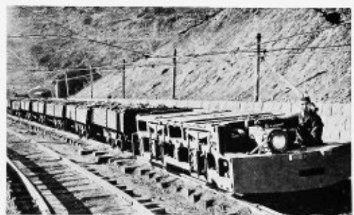
A low-design locomotive pulling a trip out of a drift mine in West Virginia. Note that the journal gibs protect the nuts on the journal boxes
