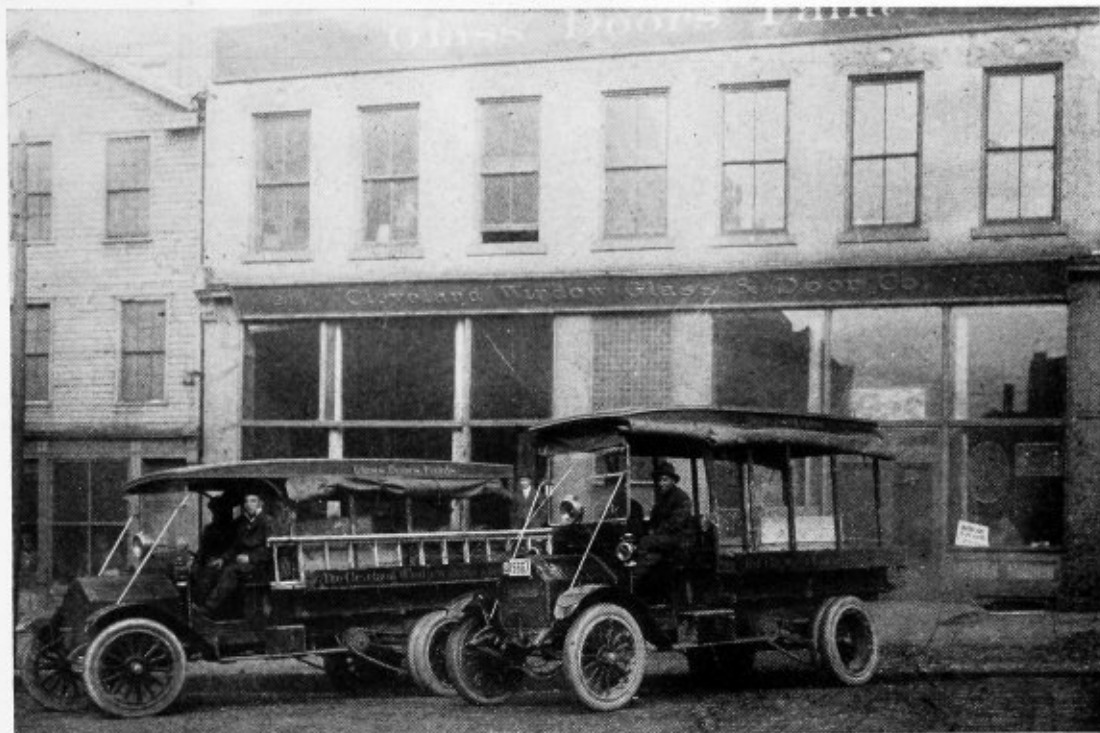
Above trucks have special rack flare-board bodies for carrying glass packed in boxes, and paints, oils, etc., inside of body proper. Equipped with pneumatic tires and demountable rims front and rear, to avoid breakage and to insure deliveries over a large territory daily. Cost of truck complete, $2,100.
