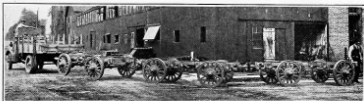
Three Trailers Being Backed Around Right Angle Corner, Guided by Man at Draw-Bar
