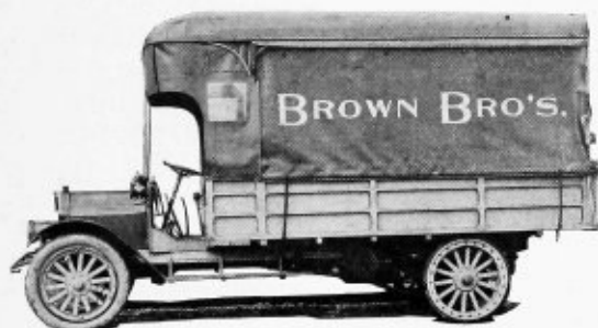
1 1/2-ton chain-drive chassis, $1800—144-in. wheelbase
