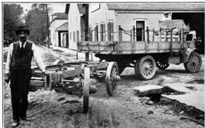
One Trailer Being Backed Around Right Angle Corner, Guided By Man at Draw-Bar
