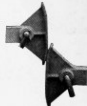
Draw-Bars Acting to Prevent Climbing in Uneven Places
