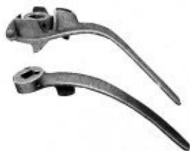
Fig. 20. New and Old Angle Cock Handle
