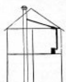
Plan C —Run vent pipe through ceiling and then into chimney or into a stove pipe.
