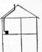
Plan D —Run vent pipe through ceiling and then up through roof as shown here.
