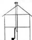
Plan A —Run the vent pipe directly into a chimney or a stove pipe, the former preferred.
