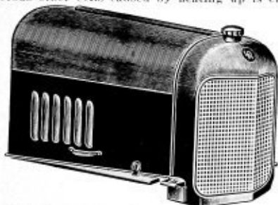
Combination "Bulldog" Radiator and Streamline Hood for 1915 and 1916 Ford Cars
