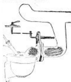
"Nycor" Accelerator and Power Adder
