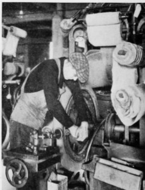
The Fabric Has Here Been Built Up Around a Core and the Operator Is Stitching Down the Plies
