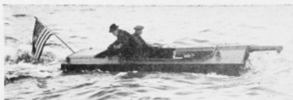
The New Battle Tank, Known as Walter Christie's Amphibious Wheel Caterpillar Tank, Recently Succeeded in Running Along the Shore and Then Crossing the Hudson River Under Its Own Power
