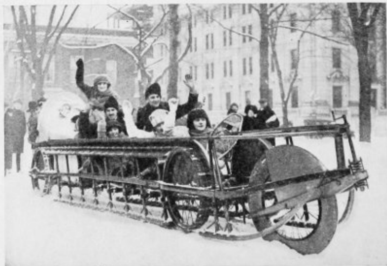
The Very Latest Idea in Sleighs Is This Motor-Driven Caterpillar Affair Propelled by a Gasoline Engine. The Sled Climbs Hills or Mountains. It Is Capable of a Speed of 45 Miles Per Hour
