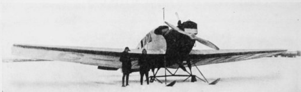
Captain Amundsen's Airplane Is Equipped with Skids for Landing on and Starting from Ice Fields. He Now Has His Ship and Air Equipment in the Arctic, Awaiting Favorable Conditions to Begin His Exploration
