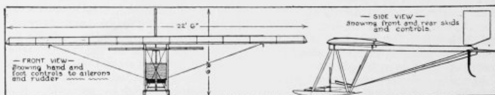
Including the Illustration on Upper Part of Page, These Three Drawings Present the Top, Front and End Views of the Sailplane. The Drawings Are Made to Scale
