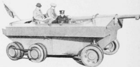
The New Battle Tank, Known as Walter Christie's Amphibious Wheel Caterpillar Tank, Recently Succeeded in Running Along the Shore and Then Crossing the Hudson River Under Its Own Power
