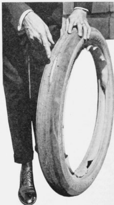
Misalignment, Locking Brakes, Wobbling Wheels and Careless Clutch Pedaling Ruins Many Tires
