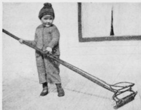
Rake Cleaner Saves One from Bending Over to Clean Teeth of Rake
