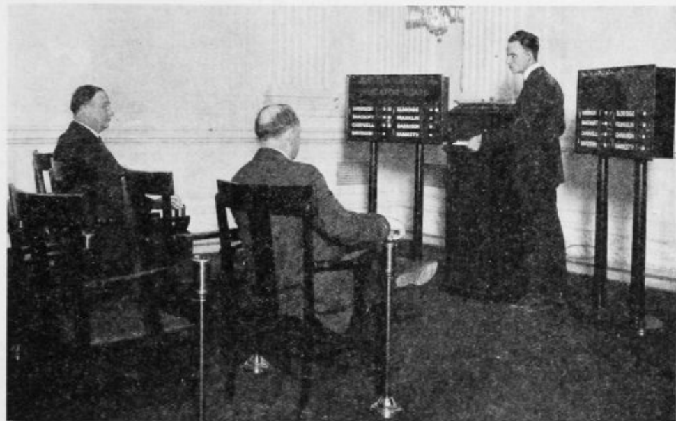
The Small Model of the Mechanical Balloting System Shows How the Big One Works. When a Congressman Presses the Button at His Seat, His Vote Is Registered and Shown by the Machine
