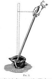
A cubic inch of mercury weighs '4908 of a pound', now, if this be multiplied by the height of the mercury column above the level of the mercury in the cap the pressure of the atmosphere can be determined ac-cording to English units. Suppose this height to be 297 inches, then  $297 \times 4908$  would be the pressure of the atmosphere under these conditions, or 1459676pounds on the square inch. Fig. 2 intertures a hypometer as supplied by makees.
