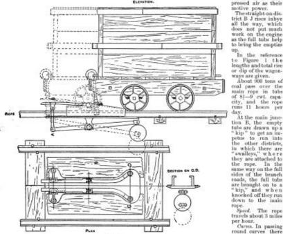
F10. 2. BEMARKS. The dotted lines drawn illustrating the "knack-off" in the elevation, show it in its untural position ; where the tab is shown in dotted lines the clip is detached, the arms having been lifted up again by the ball and lever after being depressed.
