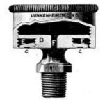
Referring to the illustration. E E is an adjustable Referring to the illustration, E E is an adjustable leather washer that can be compressed and spread by the ring C C, thereby invaring a tight joint, and prevent-ing the grease from coving out. This cup is extensively used on mining machinery. It is made of the best materials and has great advantages over iron cups which usually rust and are liable to break, thereby causing great annoyance. They are fully warranted and can be purchased of
