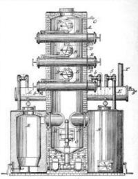
nections within the stack, as the smaller connections are liable to clog up, thus lessening the yield and causing con-siderable delay. The gas thus produced may be used by it-self or employed for enriching coal gas, or, as illustrated in Fig. 3, for carborreting water-gas.
