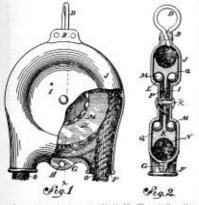
as shown, to receive two sets of balls M. These balls roll on the shoulders L of the casings and thus form circular ball bearings for the shearer. The casings may be castings, or they may be pressed into shape from sheet - etal, thus making a light, cheep and serviceable pulley block. Pric-tion is reduced to the lowest possible limit. The sheare can not bind in the casing, as the balls confine it laterally well as centrally
