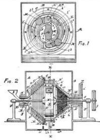
greater diameters, and having lugs and eyes for suitable bind-ing bolts as shown. These rings are separated by distance biers of suitable thickness to make the desired mesh. A period wire screen F<sup>2</sup> surrounds the ring screen E and screes to grade the material passing through it. Stuff which passes both screens falls out into the case A and passes out the look of, and that which passes the rings out all between the partitions shown, and out through
