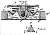
in Fig.2. The ribs which connect the hub d of the valve sext, to the rim  $d^4$ , are notched to suit the under side of the valve. The V-shapad under side of the valve deflects the water both inward and outwardly, making its passage easier than with a flat valve. The valve cannot become cocked, because the methods in the sent ribs help to guide it to its proper sent at every stroke.
