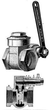
SECTION SHOWING INTERIOR CONSTRUCTION.
