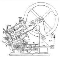
the regenerator 4. The part of the main cylinder which is exposed to fire 10, the back cylinder head 0, and the re-generator 4, are all lined with non-metallic refractory
