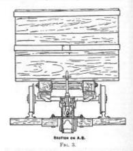
Soulleys. There being a greater tension on the full, than on the empty way, when passing "swalleys" the rope has a tendency to lift the tubs off the rails, but these "swalleys" are partially filled in on the full side. The tension not being so great on the empty way, the rown like between the rails
