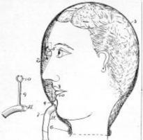
tends nearly to the floor where there is usually a layer of nir free from smoke or fumes. The top end of the base is provided with a spring clip 9 shown separately in detail, which serves to hold a sponge against the mouth and nostrils of the fireman-thus enabling him to breath in a room where the smoke would otherwise sufficient him.
