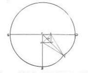
The area of D G B =  $100^{\circ} \times 3^{\circ}1416 \times \frac{3}{2} = 23,562$ square ft. The sum of the angles that can be formed around the point F = 4 right angles. The angle E F A = a right angle, and the exterior angle = 3 right angles or  $270^{\circ}$ . The line O C bisects it; then, A F C = E F C =  $135^{\circ}$ .
