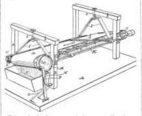
This motion is advantageous, in better spreading the ma-terial over the surface of the belt, and in keeping it worked away from the sides thereof and howard the center, result-ing in a more perfect concentration.
