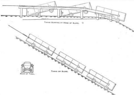
Fig. 1-Self-Londing and Self-Dumping Water-Tanks.
