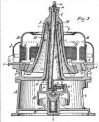
bottom of the pan, and also to throw the dust against the screens g. All that passes the screens fulls in the circu-lar chamber  $\delta_i$  and is washed out at the spout i. Centrifi-gal force also assists to keep the roller edge in good contact with the die.
