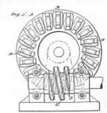
the screw or worm D with which they genr. The swiveling texth B are, by preference, enlarged or formed with shoul-ders, near their roots, bearing against ench other, as is shown, so as to distribute the string throughout the series of cogs or teeth B. The invention, though only represented as applied to the berel form of worm-wheel, is equally applicable to other
