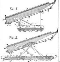
ranged to travel along these screws, and toggle-rods 25 are Fanged to travel along these screws, and loggle rods 32 are hinged to them. The naidle joint and block 29 is not at-tached to the box but merely hears under it. To dump to the rear, both screws are turned simultaneously, thus she-vating the front end of the box, which sitts on the post 23. To dump to either side, the box is first swung mound on
