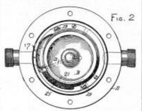
At each revolution of the crank the disc expels a volume of water equal to twice the contents of the chamber less twice the bulk of the disc and ball. The water enters at 12, passes under the chamber 13, and rises through the poet 25, and enters the chamber by a weaker-shaped opening similar to the exhaust port 16. The action of the disc is continuous and the displacement is perfectly uniform.
