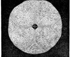
Fig. 1: Plan of mine operated by Longwall method in strong and flexible roof,
