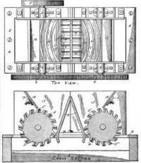
that the coal is crowded toward the middle of the rolls and away from the side housings. The groves fiseree to guide the coal past the rolls. Thus each roll is independent of its mate and crushes the coal against the plate 8, instead of the teeth of the opposite roll, as in the common type of breaker.
