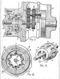
runs from the outer end of each cylinder to the bottom of the steam chest. The eight ports are arranged in a circle at exactly equal distances apart. The valve which controls the schwission and exhaust is shown in perspective in Fig. 3, and in cross section in Fig. 2.
