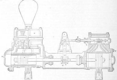
SECTIONAL VIEW OF DUPLEX BOILER PEEDER, SHOWING CAST BRASS FLANGE AND WATER CYLINDER
