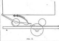
normal position, Fig. 5, a catch keeps the door of the truck closed, but should anything lift up the spring, the
