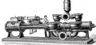
tions are cast of a high grade of composition, and the amount of this metal in the pamp end is a little over seven tons, the total weight of the engine being in the neighborhood of twelve tons.
