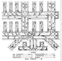
I would use to ventilate this mine a Guihal fan 12" 6" in diameter, and 5" 8" in width. It should produce 25,000 cu. ft. of air, making 210 revolutions per minute with a water-gauge of 21 inches. This ought to be suf-ficient to overcome any emergency which might occur in the mine. I would have it a force fan. Yours, etc.
