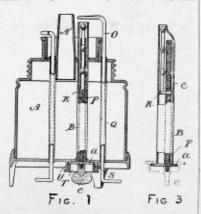
consists of a fint clongsted plate R, having a screw threaded opening, through which passes the screw red P, which is suitably switeled at its lower end in a cap-plate a, which latter rests upon the end of the nut or screw-threaded ring T, which is secured to the bottom of the oil-reservoir by
