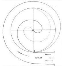
use is an outlet at c when all the air is ready to escape
