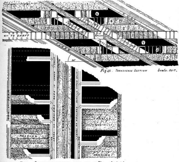
or Fig. Scale 20' Fig 46 . PLAN OF WORKINGS IN SLICE Nº 6 THE PRINCIPLES AND PRACTICE OF COAL MINING ON THE FILLAR SYSTEMS.
