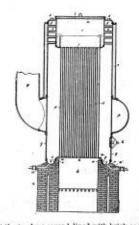
closed at the top by a cover i, lined with brick or tile m. A great number of short tubes n, run from the smoke box through the shells i and g, to the outer smoke flue or jacket
