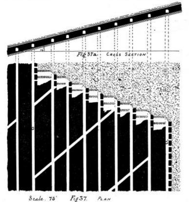
Fig. 37 is a plan, and Fig. 37a is a section on the aircourse pitch, of a system of working thick coal in France, also | for pack \*Commenced in No. 8, Vol. XI., i. c., the issue of March, 1899. Back numbers may be had by addressing The Colliery Engineer Co., Cosl Exchange, Scienton, Pa.
