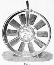
What is the anemometer's 84. See p. 163, February number of Tax Collinny Essi-Skep. 163, February number of Tax Collinny Essi-xka. The anenumeter is like a weather vane and when held up in the air-current will revolve nearly as fast as the air-current. Its pointers show how fast it does turn. does turn
