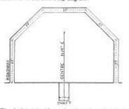
The shaft is 14' wide, and each section of roadway is 60' long and 12' wide, what would be the distance from center of shaft to center of roadway, and what would be the bearing of each section ? The center of shaft is N. 19° East. The roadway to be on North side of shaft. Yours, etc., D
