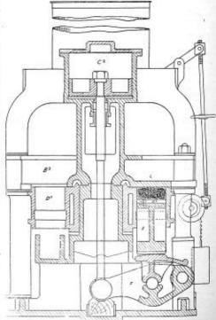
FIG. 2.-THE MANUFACTURE OF PATEST FUEL.
