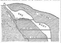
SKETCH D .- CROSS SECTION OF THE GLOBE MINE, ARIZONA dike (after Wendt). The ores as delivered at the farmace, after sorting or concentrating, will assay from 8 to 20% in copper; but as the mines become deeper,
