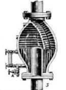
VERTICAL WHERE COURSE OF STEAM IS DOWNWARD the water being at once deposited in the lower chamber out of the current, the dry steam passes under the dia-phraga thence upward and out, being deflected by an inward extending pipe at the immediate point of out-ber
