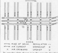
In case the pitch of seam is in the opposite direction the current should be reversed in the hout headings. Yours, etc., Winnaw KELLER.
