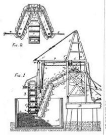
used, two of which are feeders to the main one. The frame of the main conveyor is hinged asshown in Fig. 1, and it can be swing crossways of a vessel as far as the hatchways will rollers D and D and under washing rollers P and i and it
