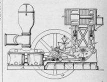
vided with a crank H, and the shaft is rotated by connect-ing rods G, which are coupled to a fourth pin B<sup>4</sup> on each beam. The valve mechanism (not shown) is driven by a "Fink" link, and is construction the working parts are mode very easy to get at, and a great economy of room is secured. The foundations required are of the plainest kind and con-sequently the expense for boildings and masonry is smaller than with other types of pumping engines.
