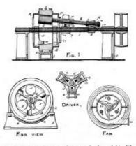
15 of sufficient tanalle strength to sustain the weight of the rolls and their shafts, are interposed between the journal boxes and the hab of the driver, to resist the downward tendency of the uppermost roll or rolls when not held outward by centrifugal force. The drivers hold the rolls to their work and prevent lateral strain which would otherwise result. The heads 16 and 17 are secured to the opposite ends of the circular die, as shown in Fig. 1, and the rock is full through the former.
