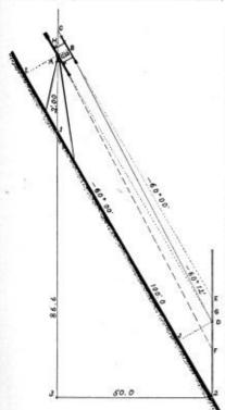
such as in lining slopes and repeating the vertical angles, which should always be done, and the angles averaged, care being taken that the rear and fore rods are vertical and that the heights to the lower telescope on both correspond. For determining the vertical heights by means of the
