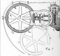
The arm B' is provided with a segmental worm-wheel E, and in journal boxes' on the fame A is journaled a worm by which engages the worm wheel E. The worm back it prolonged beyond one of its bearing. The worm back it motor whael J, which is engaged by a composition of the prolonged beyond one of its bearing and the set of the se
