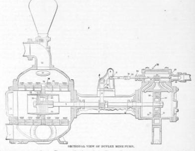
is necessary to renew them. They are fitted to the main body of the water end with ground joints, and are held in place by a heavy flarge. They are also fitted with brass valve seats, which are screwed into the valve deck with a fine tapering thread. The valve stems are of best, brass, and screw into the valve seats is a similar memory.
