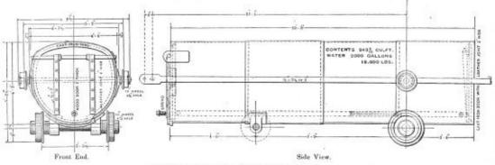
Fig. 2-Self-Londing and Self-Dumping Water-Tanks.
