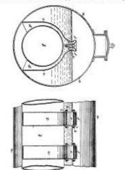
use. The tubes terminate in two sponts *f*, which shoot the mingled water and steam horizontally, thus liberating the steam from the water very thoroughly. The water passes down between the successive pairs of tubes and comes in again under the bottom ends *d*, to repeat the movement. A slight modification enables the tubes to be applied to boilers having two flues.
