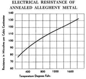
The electric resistance of copper at 68° F. is 1.72 microhms per Cm<sup>3</sup>. The electric resistance of iron at 68° F. is 12 microhms per Cm<sup>3</sup>. NOTE: To obtain the resistance in Ohms per circular mil foot multi-
